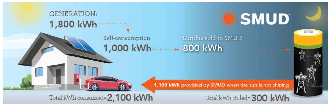
Figure 15 – Example of Flow of Electricity with a PV System and the Grid
