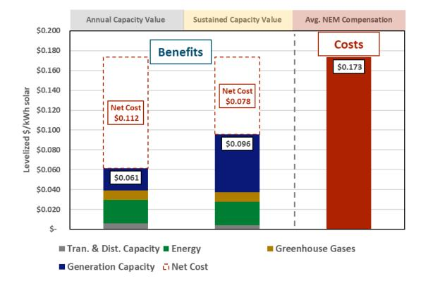
Figure 32. Value of Solar + Storage (Customer Dispatch), 2020 Installations, Sustained Capacity Sensitivity
