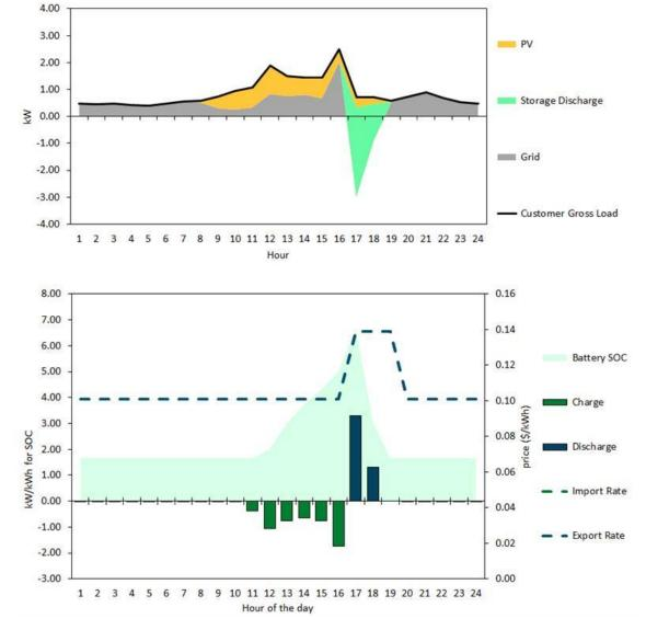
Figure 21. Sample Battery Storage Dispatch Over a Single 24-hr Period<sup>41</sup>
