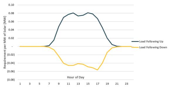
Figure 9. Average Hourly Load Following Requirements per MW of solar
