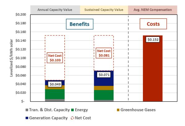
Figure 31. Value of Solar Only, 2020 Installations, Sustained Capacity Sensitivity
