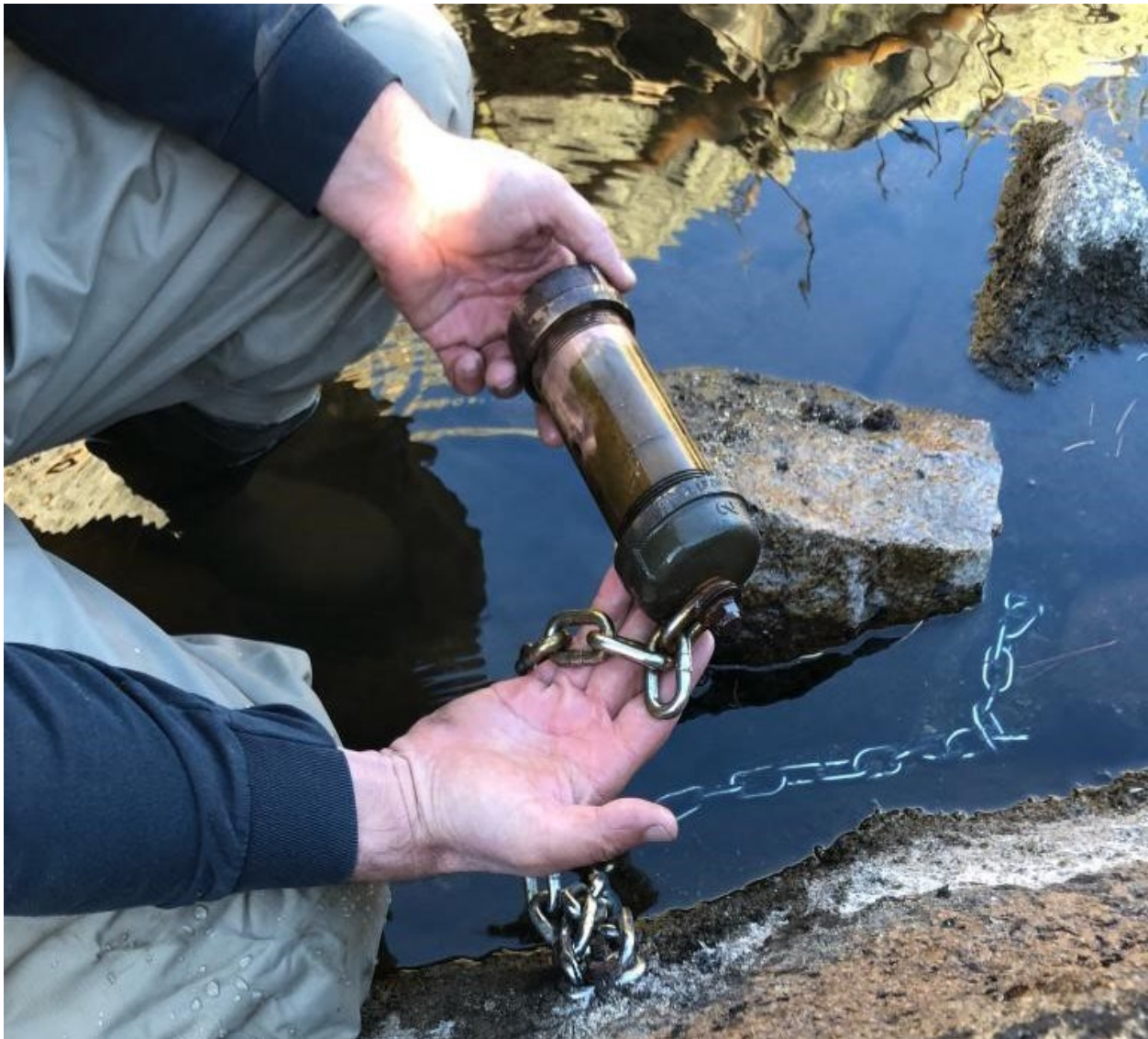
Figure 9-1. Water temperature datalogger housing, Rubicon River below confluence of Little Rubicon River.
