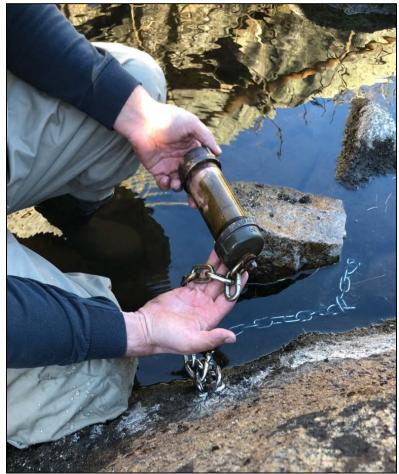
Figure 9-1. Photograph of the water temperature datalogger housing, Rubicon River below confluence of Little Rubicon River.
