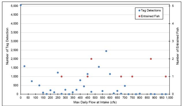
Figure 20. Robbs Peak Powerhouse intake flow (cfs), PIT tag detections, and entrained PIT tagged fish. Detections that appear on the X-axis correspond to low detection numbers, not "0" detections.
