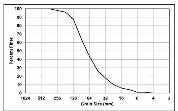
Figure Att.2-1. Bed surface gradation at the Gerle Creek Delta critical riffle
