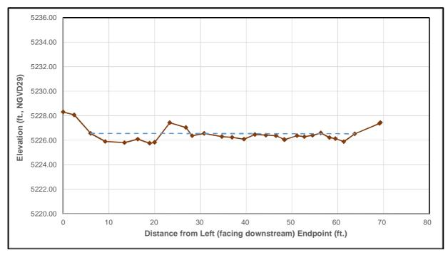
Figure 12. Surveyed cross section geometry near PCR4 (as viewed facing downstream).
