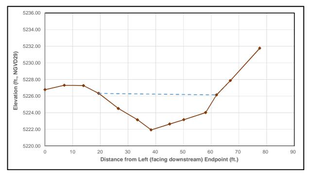
Figure 4. Surveyed cross section geometry near PCR1 (as viewed facing downstream).
