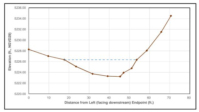
Figure 6. Surveyed cross section geometry near PCR2 (as viewed facing downstream).
