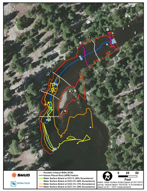
Figure 1. PCR and HPR features on the Gerle Creek delta, and water surface extents.
