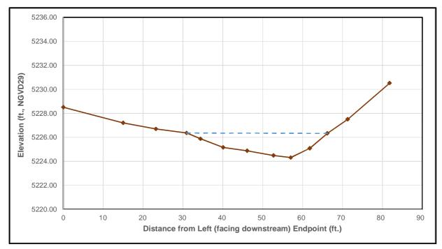
Figure 8. Surveyed cross section geometry near PCR3 (as viewed facing downstream).
