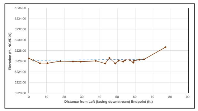
Figure 10. Surveyed cross section geometry near HPR1 (as viewed facing downstream).
