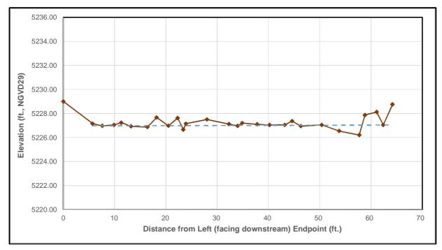
Figure 14. Surveyed cross section geometry near HPR2 (as viewed facing downstream).
