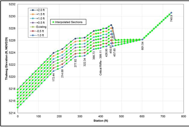
Figure 10. Comparison of channel thalweg profiles for simulated aggradation and degradation
