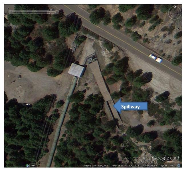
Figure 2. Flow diversion channel above Robbs Peak Powerhouse used during construction but not used as an emergency spillway.
