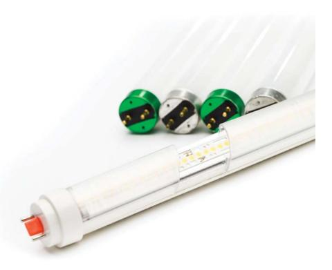
ended power inputs use both lamp sockets for power and mechanical support. The power is typically 110-277VAC for both formats and requires bypassing the fluorescent ballast and re-wiring the lamp sockets. Regardless of the lamp type, SMUD recommends replacing the lamps sockets during installation.
