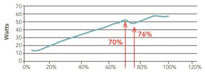
This popular dimming ballast consumes more power when dimmed to 70% than it does at 76% (due to cathode heating).
