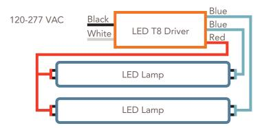
Note: Sample wiring diagram. Consult with TLED manufacturer for specific wiring instructions..
