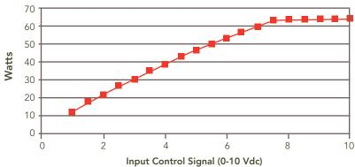
This commonly used ballast has a deadband from 7.5V – 10V (lights won't provide energy savings until dimmed approximately 25%).
