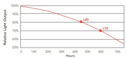
Typical life of a LED: L70 = when the LED loses 30% of its lumen output. L80 = when the LED loses 20% of its lumen output.
