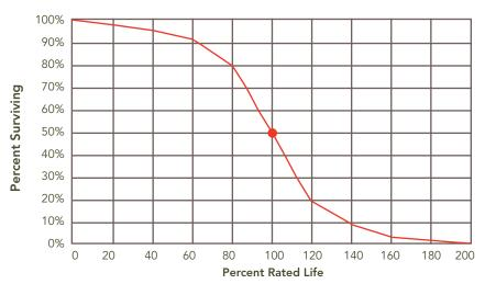
Typical life of a lamp (non-LED): half of the lamps fail at the published rated life. i.e. 36,000 hours (lamp life varies with 3 hour or 12 hour starts)
