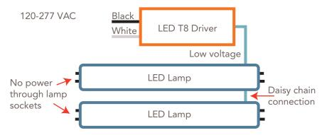
Note: Sample wiring diagram. Consult with TLED manufacturer for specific wiring instructions.
