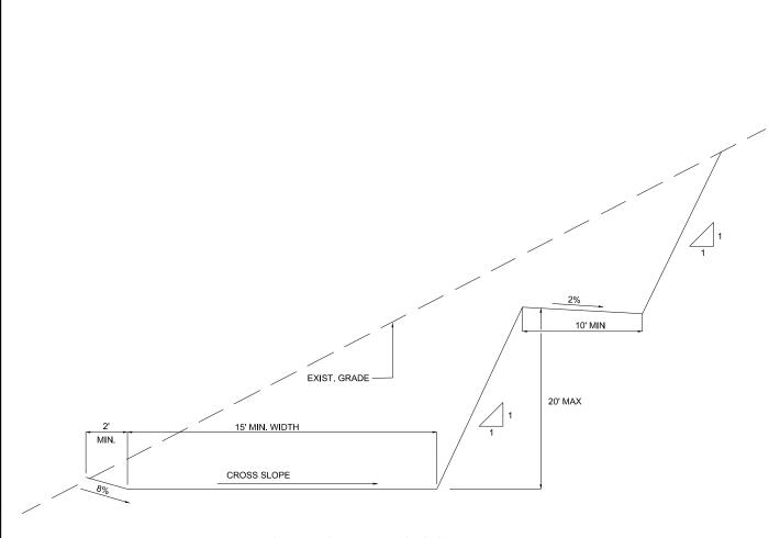
TYPICAL FULL CUT WITH BENCH SECTION ALL EXIST. GRADE CROSS SLOPES GREATER THAN 80% AND WHERE REQUIRED BY ENGINEER
