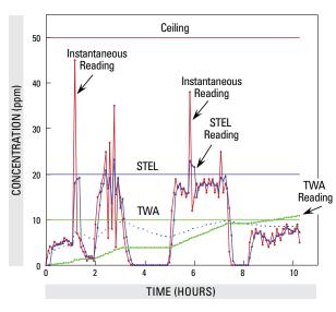
FIGURE 4.2.1. Exposure limit illustration: TWA vs. running average
