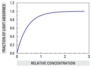
FIGURE 2.6.2. Fraction of light absorbed vs. concentration showing linear response at low concentrations and saturation by total absorbance at very high concentrations
