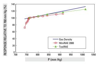
FIGURE 3.3.2. Pressure dependence for two PIDs
