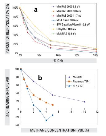
FIGURE 3.2.4. Effect of methane on the response of various PIDs with 10.6 eV lamps. Data for the Photovac TIP-1 and HNU-101 are adapted from Nyquist et al. (1990)
