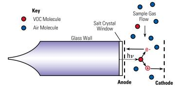
FIGURE 2.1.1. General schematic of a PID sensor
