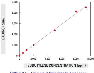
FIGURE 2.6.6. Example of linearized PID response
