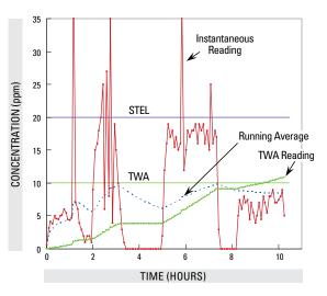
FIGURE 4.2.3. Exposure limit illustration: TWA vs. running average
