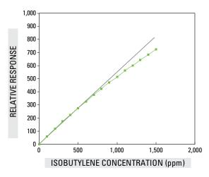
FIGURE 2.6.4. Raw response of a MiniRAE 2000 PID with 10.6 eV lamp as a function of isobutylene concentration in the high ppm range
