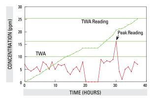
FIGURE 4.2.4. Exposure limit illustration: TWA exceeds peak
