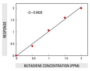
FIGURE 4.19.1. UltraRAE butadiene response in the presence of 100 ppm hexane using a RAE-Sep butadiene tube and 9.8 eV lamp Table 4.19.1 lists the apparent response to a variety of compounds that may interfere in benzene measurements. Thus, appropriate filtering can provide selective measurements in the presence of large excesses of other responding compounds in certain applications.
