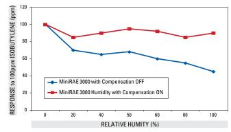
FIGURE 3.2.7(a). Effect of humidity PID response
