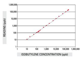
FIGURE 2.6.3. Response of a ppbRAE PID with 10.6 eV lamp as a function of isobutylene concentration in the ppb to middle ppm range
