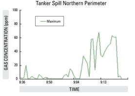
FIGURE 4.3.4. Datalogged PID response at a HazMat incident perimeter
