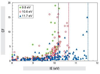
FIGURE 3.0.1. PID correction factor vs. compound ionization energy for various lamps
