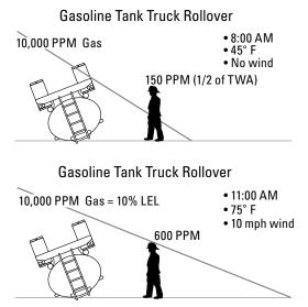
FIGURE 4.3.3. Perimeter variation due to changing weather conditions
