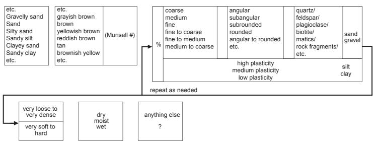
e.g. D Silty sand; light yellowish brown (2.5Y 6/3); 80% fine to medium, subangular, quartz/feldspar sand; 15% low plasticity silt; trace fine, subangular, rock fragments; gravel; dense; dry
