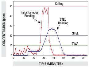
FIGURE 4.2.2. Exposure limit illustration: STEL
