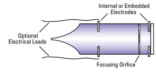
FIGURE 2.3.1. Cross-section view of DC discharge lamp
