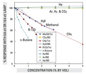
FIGURE 3.2.5. Effect of matrix vapors on MiniRAE PID Response to 50 ppm toluene, 100 ppm IBE, or butane self-quenching. All experiments except those of H<sub>2</sub>, He, Ar, and butane had pure air as the balance gas. The others had N<sub>2</sub> as the balance
