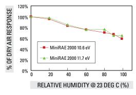
FIGURE 4.13.1. Response to test gas with clean sensor
