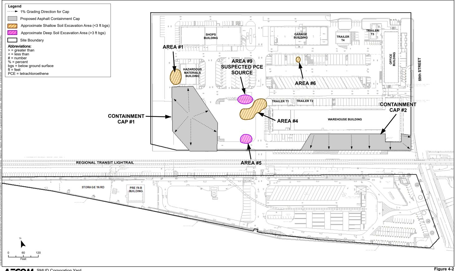
Alternative 3 - Limited Soil Excavation/Off-Site Disposal, Soil Containment/Capping-in-Place, and Land Use Controls
