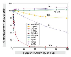
FIGURE 3.2.6. Effect of various gases on MiniRAE PID response with a 10.6 eV lamp. The 9.8 eV lamp has similar effects with CH<sub>4</sub> and O<sub>2</sub>
