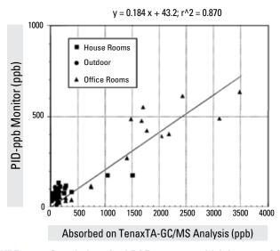
FIGURE 4.11.1. Correlation of ppbRAE response with laboratory GC/MS
