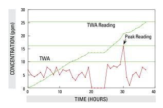
FIGURE 4.2.4. Exposure limit illustration: TWA exceeds peak
