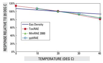
FIGURE 3.3.1. Effect of temperature on three PIDs
