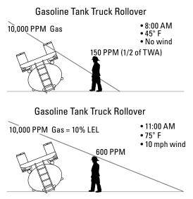
FIGURE 4.3.3. Perimeter variation due to changing weather conditions
