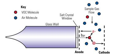
FIGURE 2.1.1. General schematic of a PID sensor
