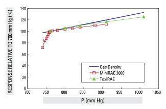
FIGURE 3.3.2. Pressure dependence for two PIDs
