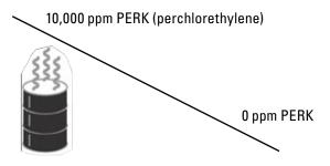
FIGURE 4.3.2. Concentration gradient from a vapor source
