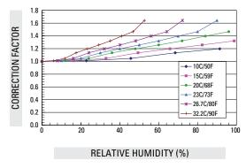
FIGURE 3.2.9. Correction factors for humidity vs. temperature for MiniRAE 2000
