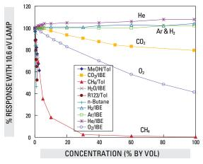
FIGURE 3.2.6. Effect of various gases on MiniRAE PID response with a 10.6 eV lamp. The 9.8 eV lamp has similar effects with CH<sub>4</sub> and  $0_2$
