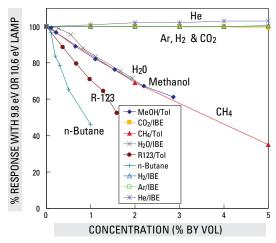
FIGURE 3.2.5. Effect of matrix vapors on MiniRAE PID Response to 50 ppm toluene, 100 ppm IBE, or butane self-quenching. All experiments except those of  $\rm H_2$ , He, Ar, and butane had pure air as the balance gas. The others had  $\rm N_2$  as the balance
