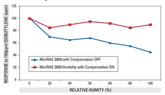
FIGURE 3.2.7(a). Effect of humidity PID response
