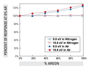
FIGURE 3.2.7. Comparison of argon effect on PID response to IBE in air vs. N<sub>2</sub>
