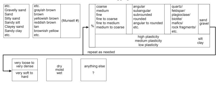
e.g. D Silty sand; light yellowish brown (2.5Y 6/3); 80% fine to medium, subangular, quartz/feldspar sand; 15% low plasticity silt; trace fine, subangular, rock fragments; gravel; dense; dry e.g. D Sandy clay; strong brown (7.5YR 5/6); 85% low plasticity clay; 15% fine, angular, quartz sand; stiff; moist
