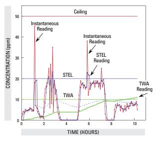
FIGURE 4.2.1. Exposure limit illustration: TWA vs. running average
