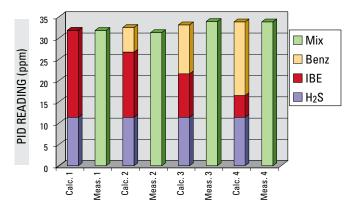
FIGURE 2.7.1. Additivity of PID response in mixtures
