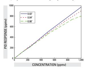
FIGURE 2.4.1. Effect of sensor light pathlength on response linearity
