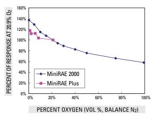
FIGURE 3.2.3. Effect of oxygen on MiniRAE PID response to 100 ppm isobutylene with an 11.7 eV lamp
