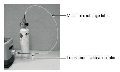
FIGURE 4.14.1. Connection of moisture exchange tube to gas cylinder and open calibration tube
