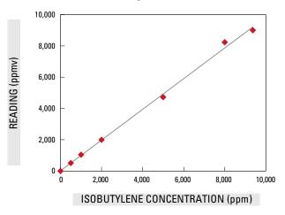
FIGURE 2.6.6. Example of linearized PID response
