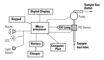
FIGURE 2.5.1. Overall PID instrument schematic
