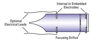
FIGURE 2.3.1. Cross-section view of DC discharge lamp
