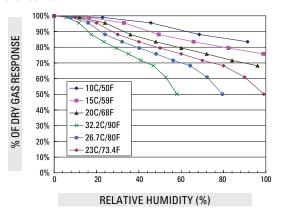
FIGURE 3.2.8. Calculated PID humidity effect curves vs. temperature for MiniRAE 2000
