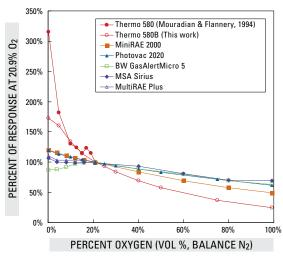
FIGURE 3.2.1. Effect of oxygen on various PID responses to 100 ppm isobutylene
