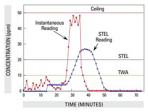
FIGURE 4.2.2. Exposure limit illustration: STEL
