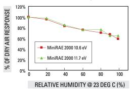
FIGURE 4.13.1. Response to test gas with clean sensor
