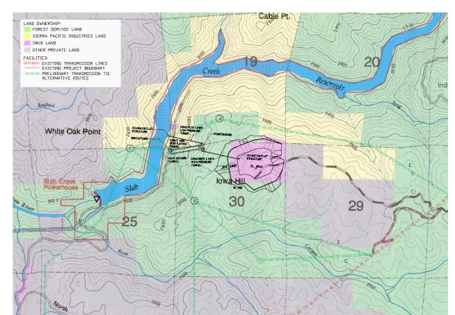
Figure 4.0 Possible Transmission Line Routes for the Proposed Iowa Hill Development
