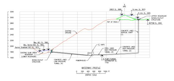
Figure 3.0 Cross-Section of the Proposed Iowa Hill Project
