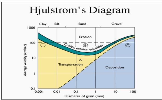
Figure 3.3.3-1. Hjulstrom Diagram delineating critical velocities for erosion.
