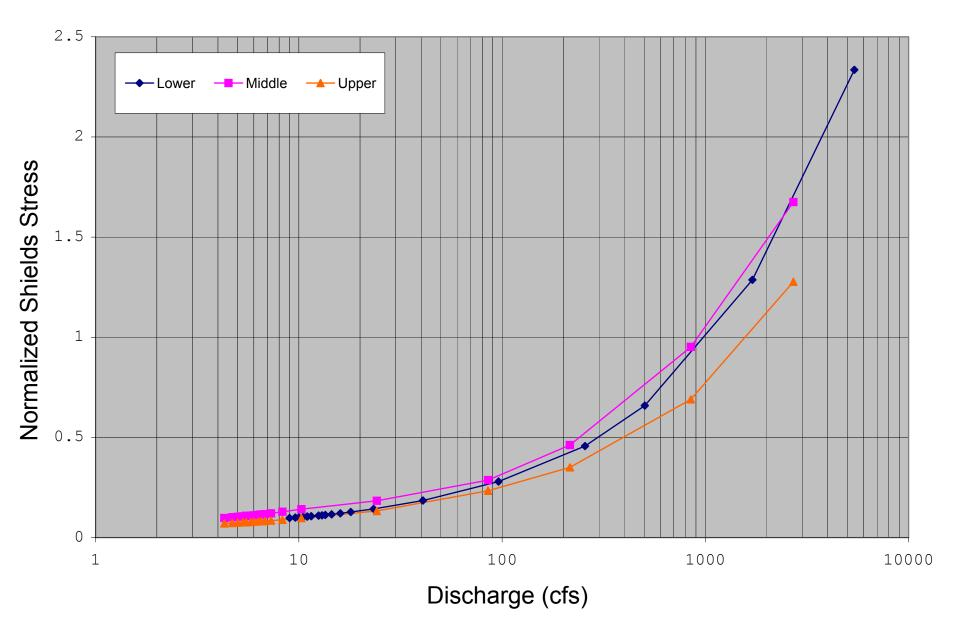
Figure N-8: Estimated Shields stress rating curve for the Robbs Peak Dam Reach Site.
