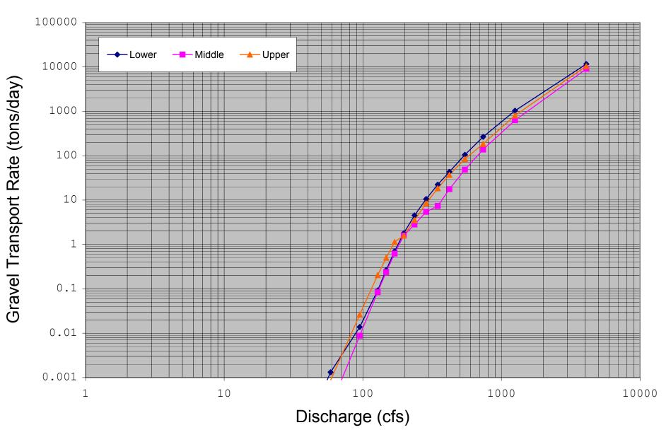
Figure N-1: Estimated bedload transport rating curve for the Rubicon Dam Reach Site.
