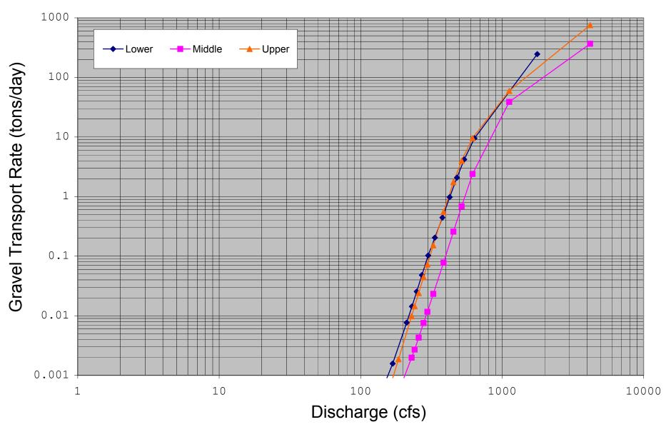
Figure N-11: Estimated bedload transport rating curve for the Ice House Dam Reach Lower Site.
