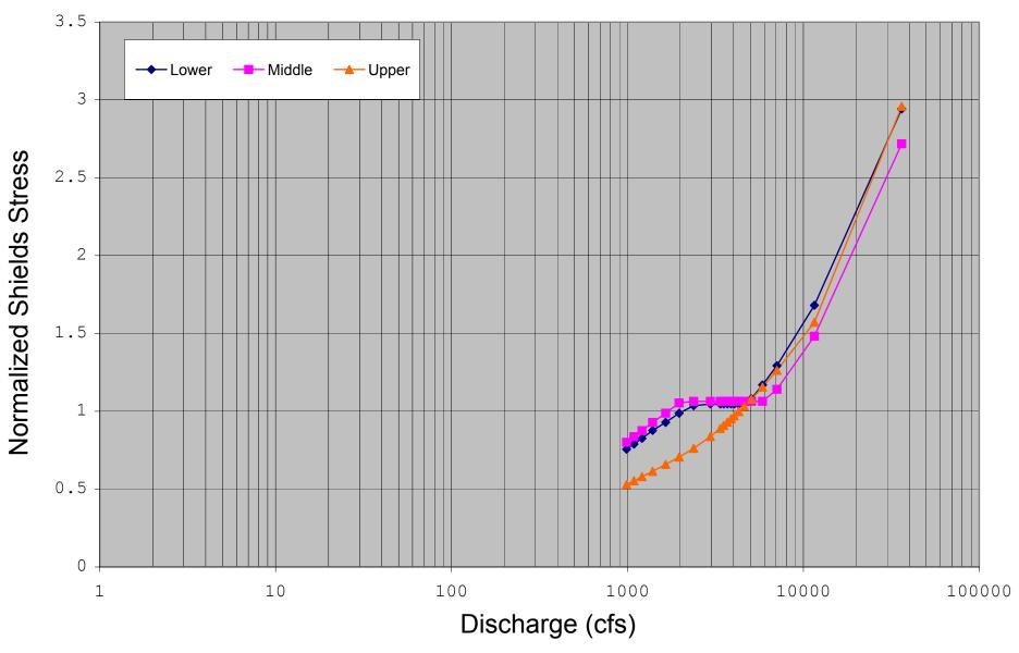
Figure N-14: Estimated Shields stress rating curve for the Reach Downstream of Chili Bar, Upper Coloma Study Site.
