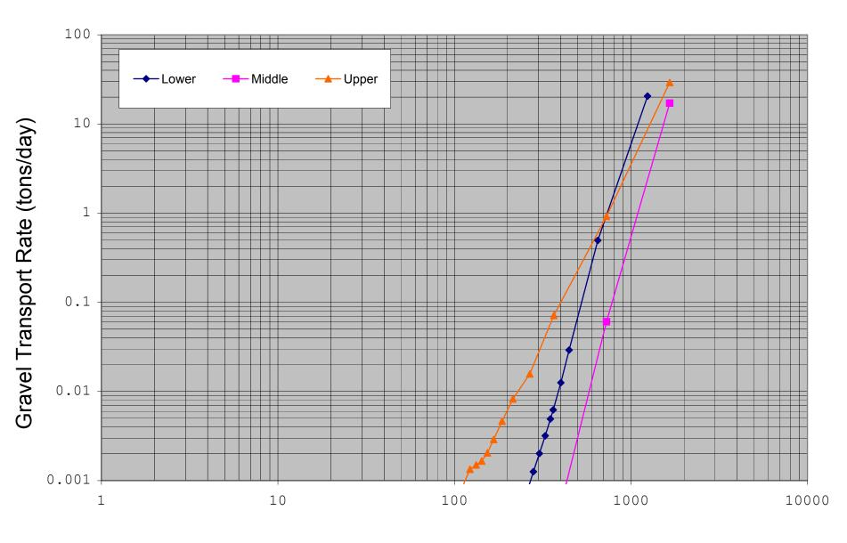
Figure N-5: Estimated bedload transport rating curve for the Loon Lake Dam Reach Lower Site.
