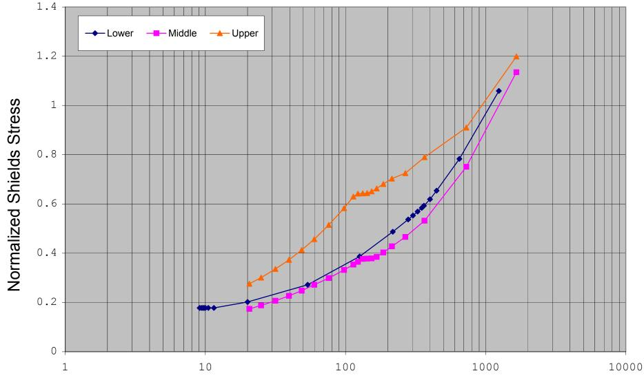
Figure N-6: Estimated Shields stress rating curve for the Loon Lake Dam Reach Lower Site.
