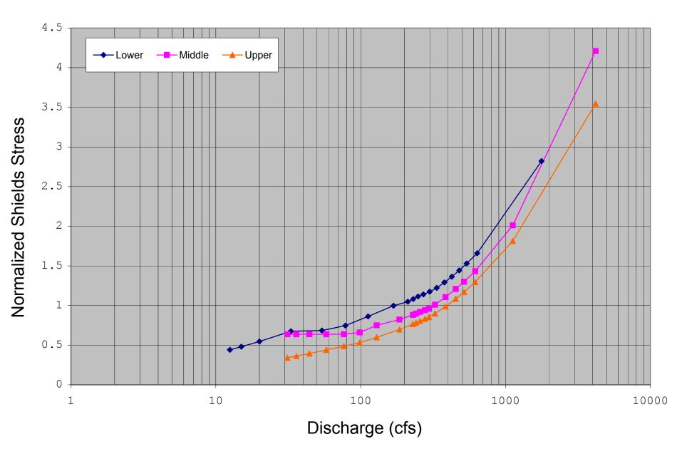
Figure N-10: Estimated Shields stress rating curve for the Ice House Dam Reach Upper Site.
