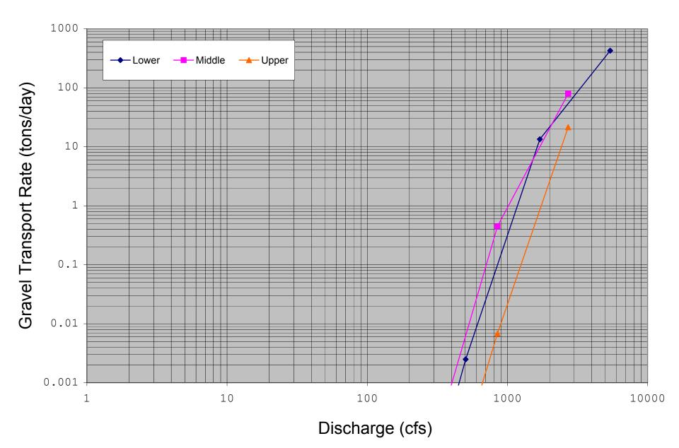
Figure N-7: Estimated bedload transport rating curve for the Robbs Peak Dam Reach Site.
