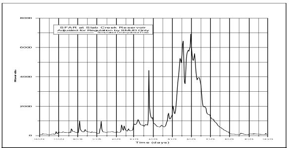
Figure 4.8-1. Synthesized unimpaired hydrograph for the SFAR October 1974 through September 1975.
