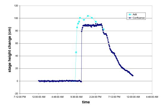
Figure G3.3-1. Change in stage height at the Adit and Confluence sites on Silver Creek on September 15, 2004. Flows of 600 cfs were released from Camino Dam at approximately 6:10 a.m.
