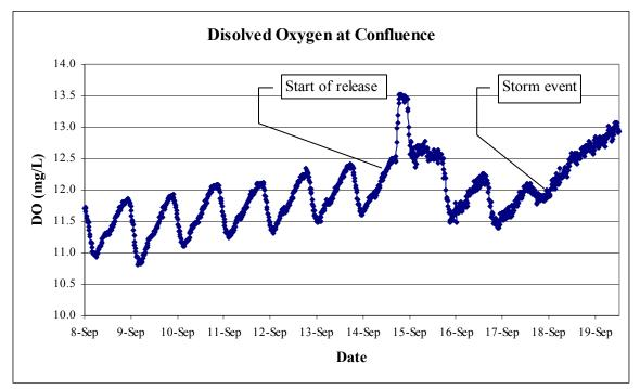
Figure G4.1-9. Dissolved oxygen concentrations measured at the Confluence Site from September 8 through September 20, 2004.
