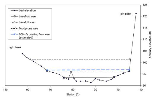
Figure G3.3-2. Estimated water surface elevation, based on estimated stage change, at the Adit Site, Camino Dam Reach. Water surface elevations are further explained in the *Channel Morphology Technical Report*.
