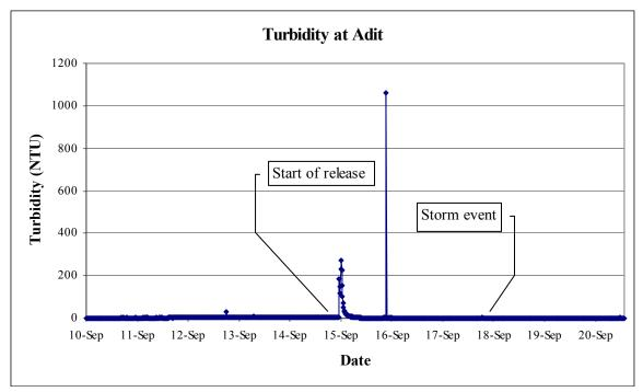
Figure G4.1-5. Turbidity measured at the Adit Site from September 10 through September 20, 2004.
