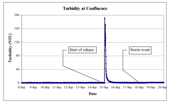
Figure G4.1-6. Turbidity measured at the Confluence Site, from September 8 through September 20, 2004.
