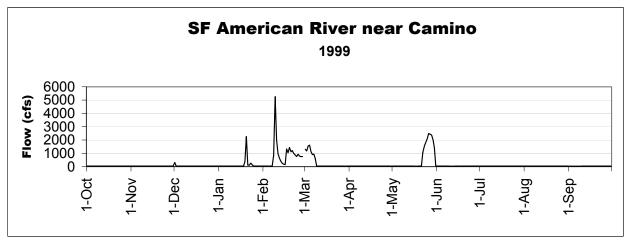
Figure 4.8-2. Regulated hydrograph for the SFAR, October 1998 through September 1999.
