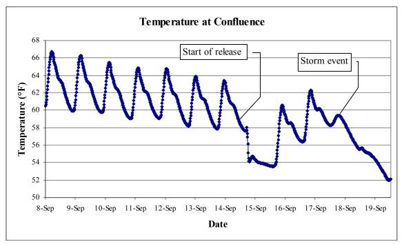
Figure G4.1-3. In-Situ water temperatures recorded at the Confluence Site September 8 through September 20, 2004.
