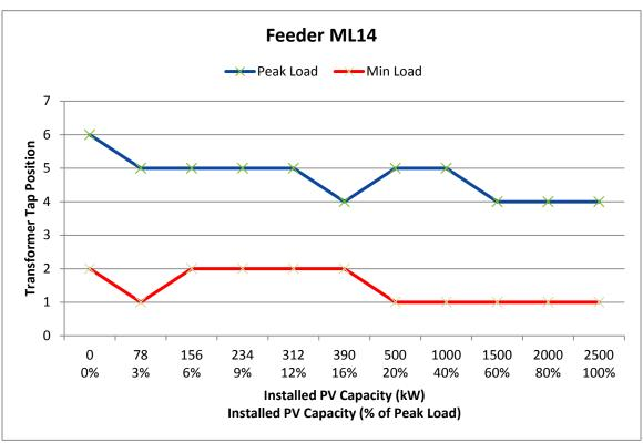
Figure 3-19. ML12 (top) and 14 (bottom) transformer tap position vs. PV penetration %
