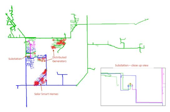
Figure 3-7. Feeder layout for AC1, AC2, and AC3 (AC1 in blue, AC2 in green, and AC3 in red)
