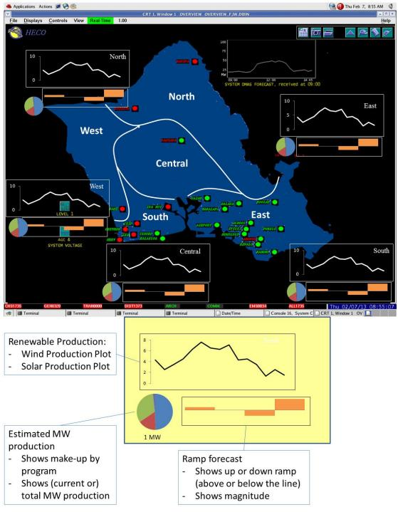
Figure 5-14. Prototype of regional forecasts and ramp statistics (source: Siemens and HECO)
