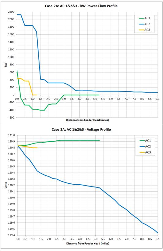
Figure 3-10. AC1, AC2, and AC3 power flow and voltage profiles for Scenario 2A
