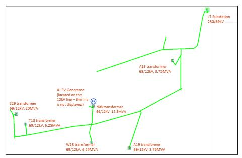
Figure 3-13. L7 feeder one-line diagram
