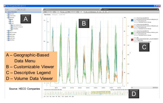
Figure 5-6. Perspective view of renewable data and customizable data-handling features (A-D)
