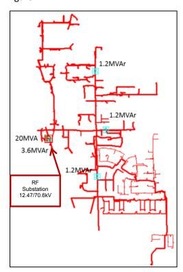
Figure 3-14. RF one-line diagram
