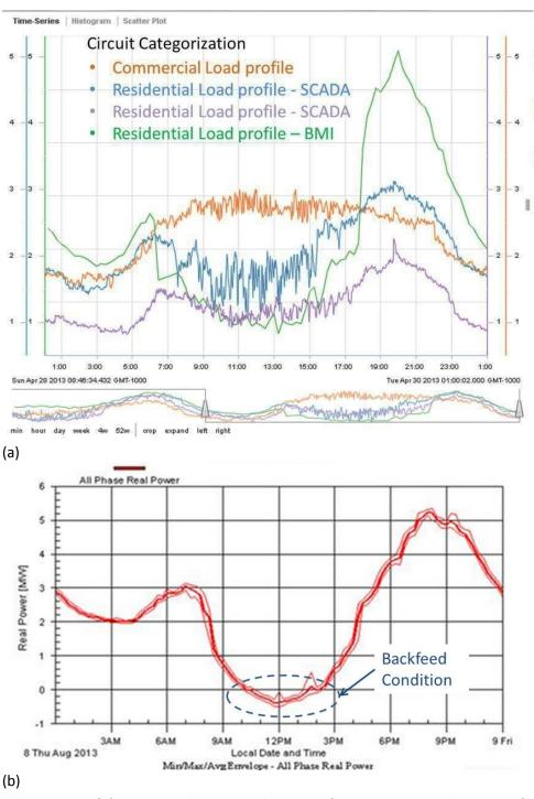
Figure 5-8. (a) Visual confirmation of mid-day (10 a.m. to 2 p.m. for Hawaii) impact of PV on different types of feeder loads (commercial, residential, industrial or combined) at different resolutions with different monitoring devices (SCADA and Basic Measuring Instrument power monitoring devices) and (b) measured backfeed condition (source: HECO)
