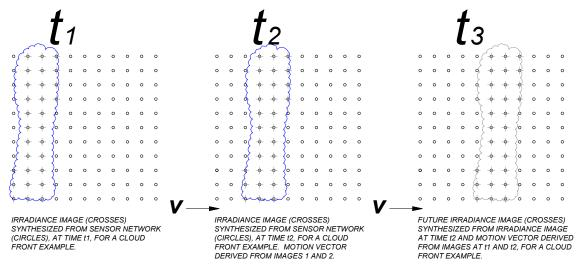
Figure 6-12. Example of initial methodology for 0-3 hour irradiance forecast: Ground Level Irradiance Velocity Vector Recognition
