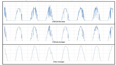
Figure 3-1. MECO irradiance full week, three time increments
