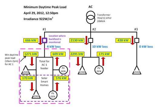
Figure 3-8. AC1 power flows for minimum daytime peak conditions
