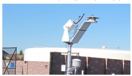
Figure 6-8. One of the four RSRs with a PSP installed
