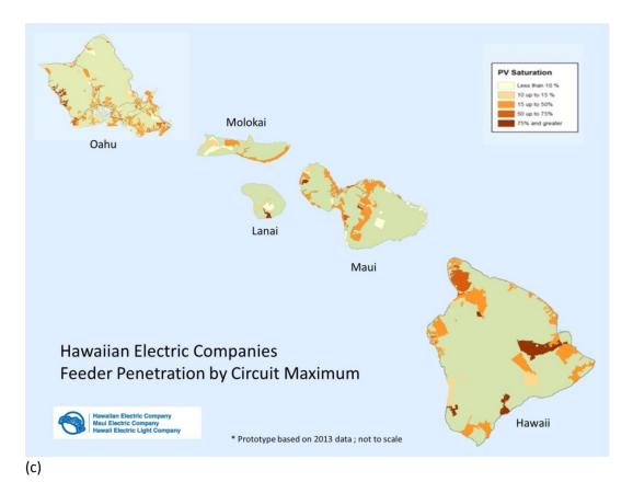
Figure 5-11. New 5-tone LVM with (a) percentage penetration of circuit maximum,
