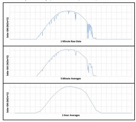
Figure 3-2. MECO irradiance select day, three time increments
