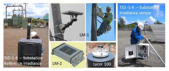
Figure 5-3. Examples of solar monitoring devices deployed in Hawaii and California
