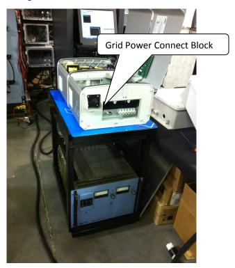
Figure 4-4. Inverter and DC power supply
