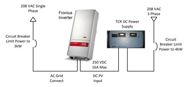
Figure 4-3. Power wiring diagram
