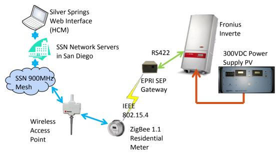
Figure 4-1. Testing at SMUD facility
