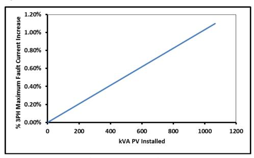
Figure 3-24. Maximum % fault current increase for WO 3
