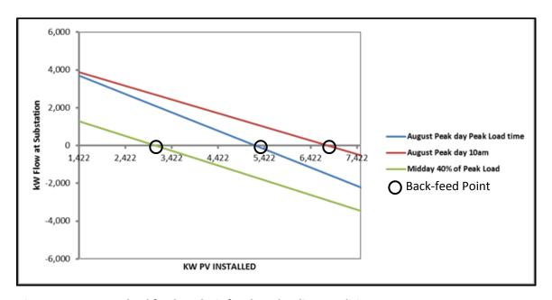
Figure 3-23. WO 3 backfeed analysis for three loading conditions
