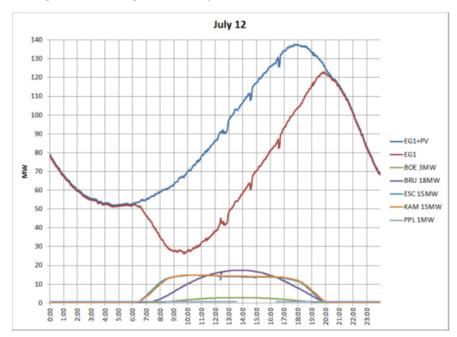
Figure 3-4. July 2012 load curve for EG
