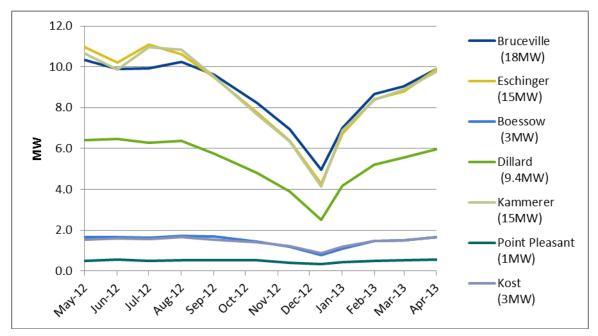
Figure 6-18. Average monthly measured power per FIT site
