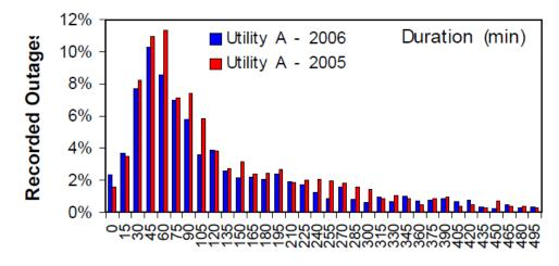
Figure 2-1 Recorded Outage Durations for two U.S. Utilities (NREL 2009)
