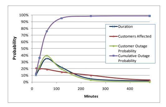
Figure 2-2 SMUD System 2008 – Base Case – Customer Perspective Outage Calculation
