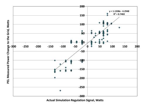
Figure 36 Measured Power Differences Versus Simulated Regulation Signal Power Differences.
