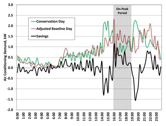
Figure 23 Average Air Conditioning Unit Profiles and Savings on Conservation Days.
