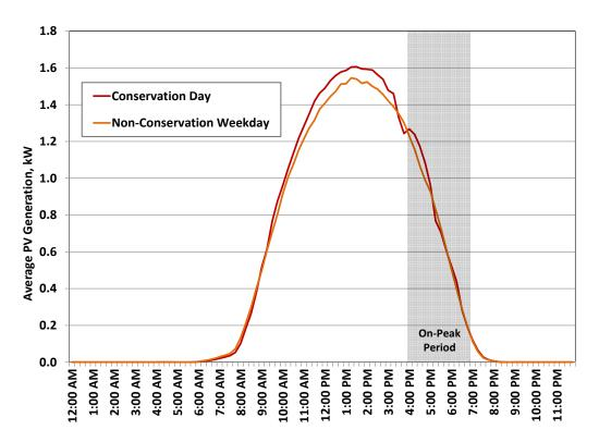
Figure 16 PV Power Generation Profiles for Conservation and Non-Conservation Days.
