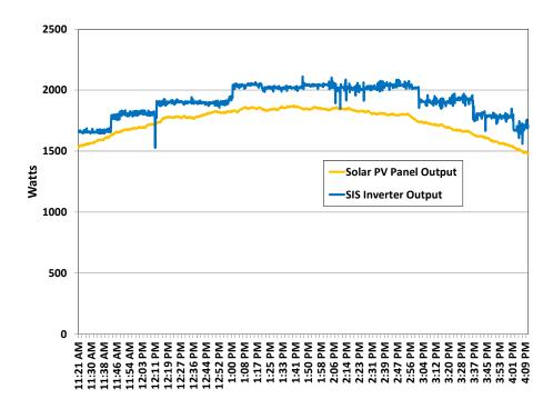
Figure 33 Example of the Inverters 100 Watt Step Minimum Change.
