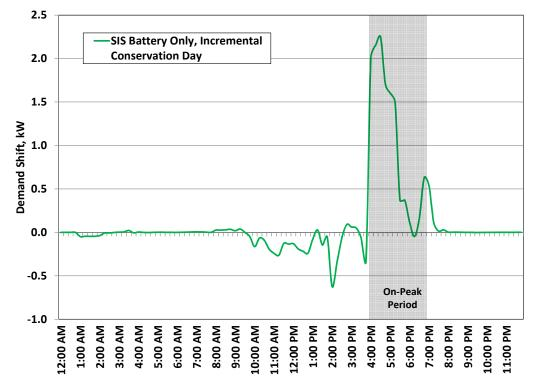
Figure 19 Average House SIS Battery Only Load Shifting Demand Profile for Incremental Conservation Days.
