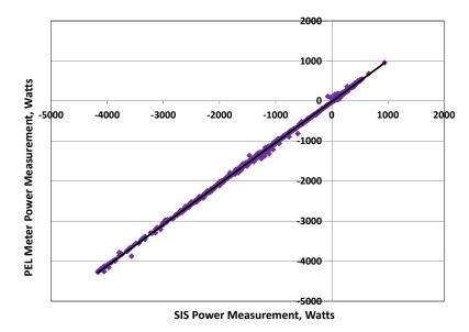
Figure 37 House Panel (to Grid) Power Measurement Comparison of Two Meters.
