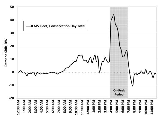
Figure 29 Total Fleet IEMS Load Shifting Profile for an Average Conservation Day.
