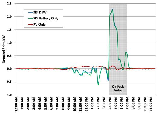
Figure 20 Comparing Incremental Load Shifting Demand Profile for Conservation Days.
