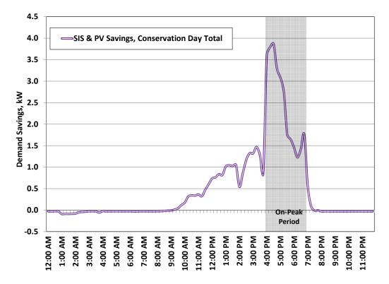
Figure 15 Average House SIS & PV Total Load Shifting Savings Profile for Conservation Days.
