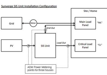
Figure 5 Arrangement of Power Meters around SIS Installed by ADM at Three Houses.
