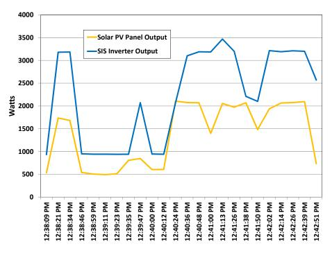
Figure 31 Largest SIS Power Output Changes Observed During "Send to Grid PV Only" Mode.
