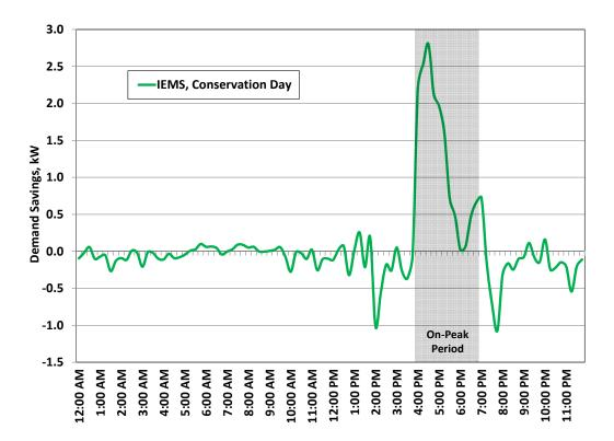
Figure 11 Average House IEMS Load Shifting Savings Profile for Incremental Conservation Days.
