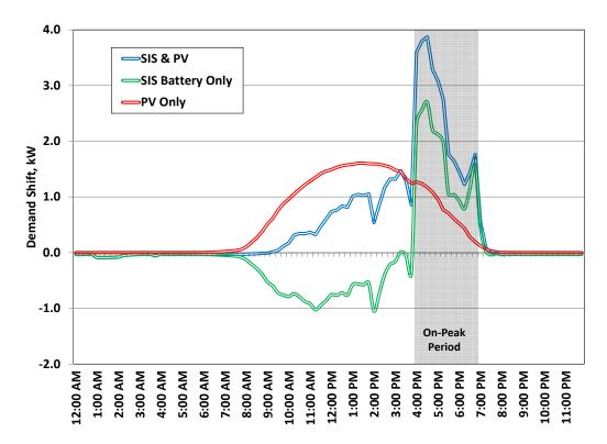
Figure 22 Comparing Total Load Shifting Demand Profiles for Conservation Days.
