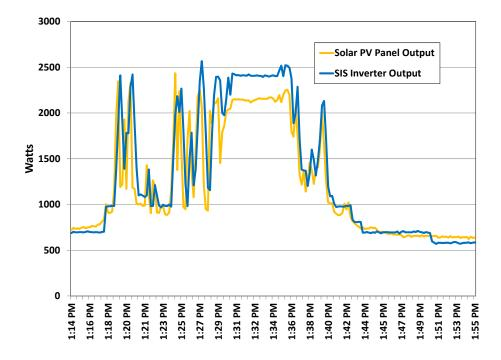
Figure 32 Rapid Changes in PV and SIS Power Outputs During Partly Cloudy Day.
