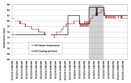
Figure 24 PCT Set Point Changes at 2:00 p.m., 4:00 p.m., and 7:00 p.m. for One Home on Sept. 12<sup>th</sup> a Conservation Day.
