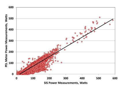
Figure 38 Critical Load Panel Power Measurement Comparison of Two Meters.
