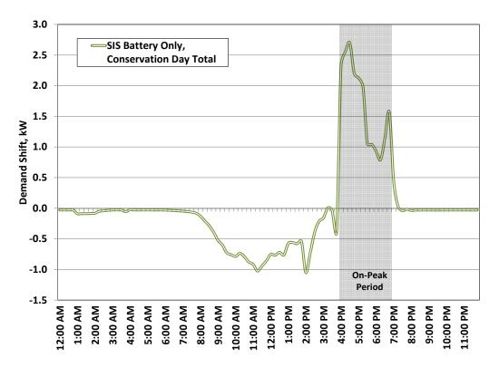
Figure 21 Average House SIS Total Load Shifting Demand Profile for Conservation Days.
