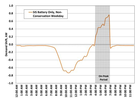
Figure 17 SIS Battery Only Load Shifting Demand Profile for Non-Conservation Weekdays.
