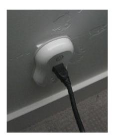
Figure 4 Modlet Plugged into Wall Outlet with Appliance Cord.
