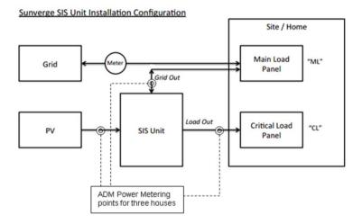
Figure 30 Configuration of Power Meters Installed by ADM at Three Houses.
