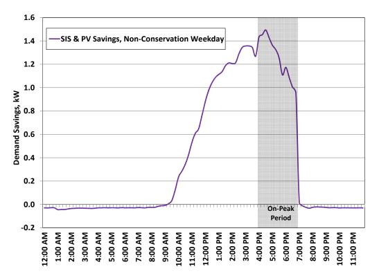
Figure 13 SIS & PV Load Shifting Savings Profile for Non-Conservation Weekdays.
