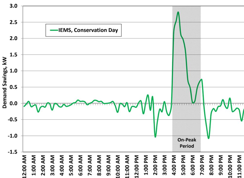
Figure 11 Average House IEMS Load Shifting Savings Profile for Incremental Conservation Days.
