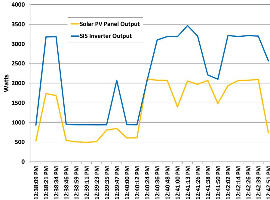
Figure 31 Largest SIS Power Output Changes Observed During “Send to Grid PV Only” Mode.
