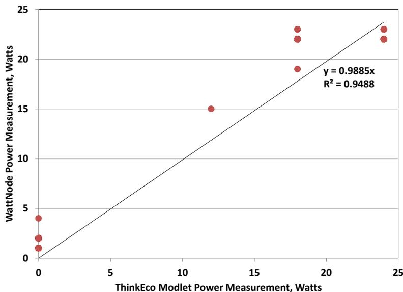
Figure 42 Comparison of WattNode versus Modlet Power Measurements of a Fan.
