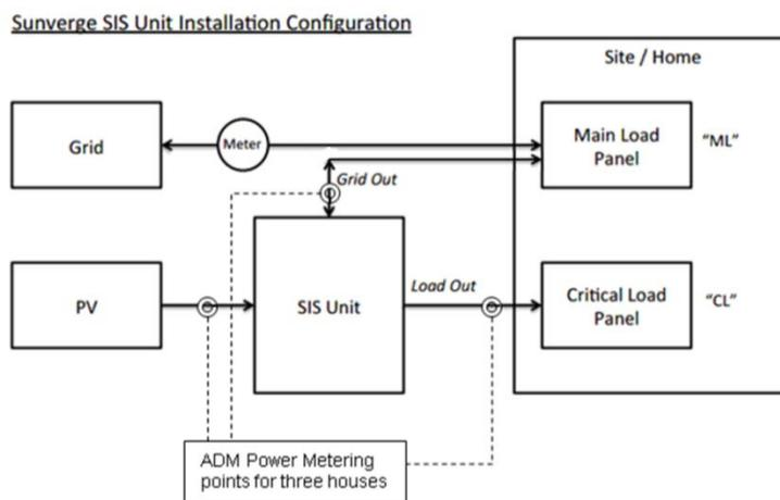
Figure 5 Arrangement of Power Meters around SIS Installed by ADM at Three Houses.
