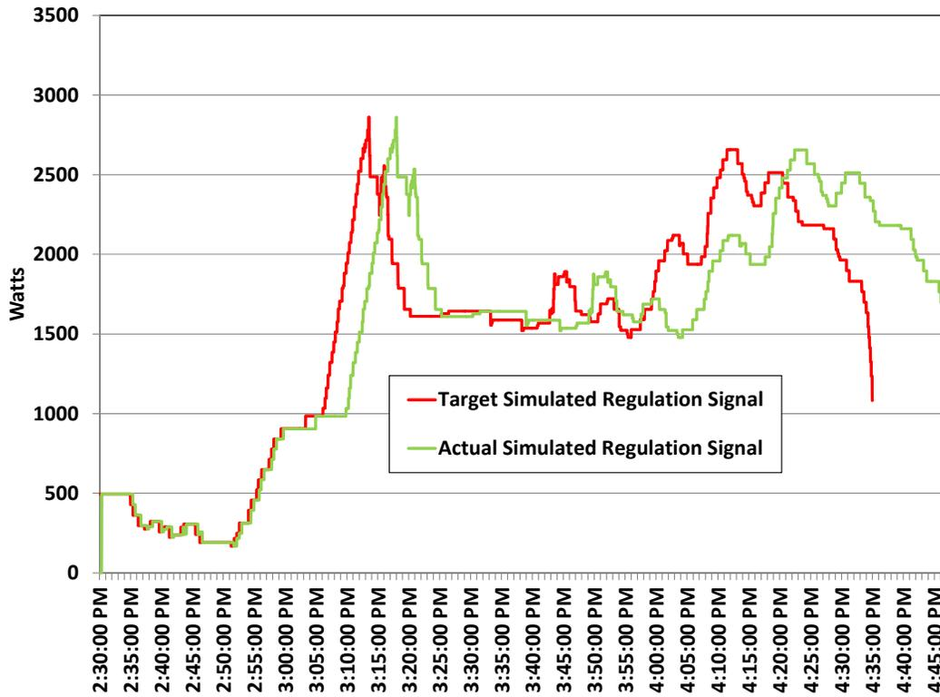
Figure 34 Target and Actual Simulated Regulation Signal.
