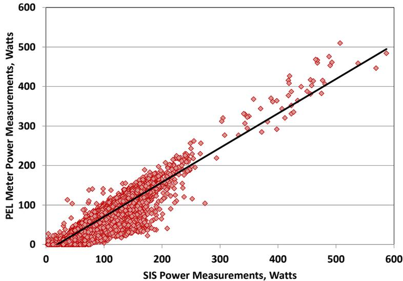
Figure 38 Critical Load Panel Power Measurement Comparison of Two Meters.
