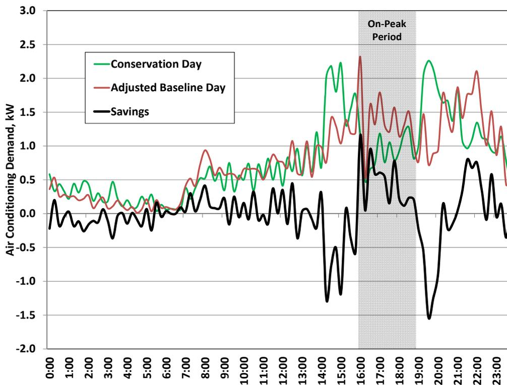
Figure 23 Average Air Conditioning Unit Profiles and Savings on Conservation Days.
