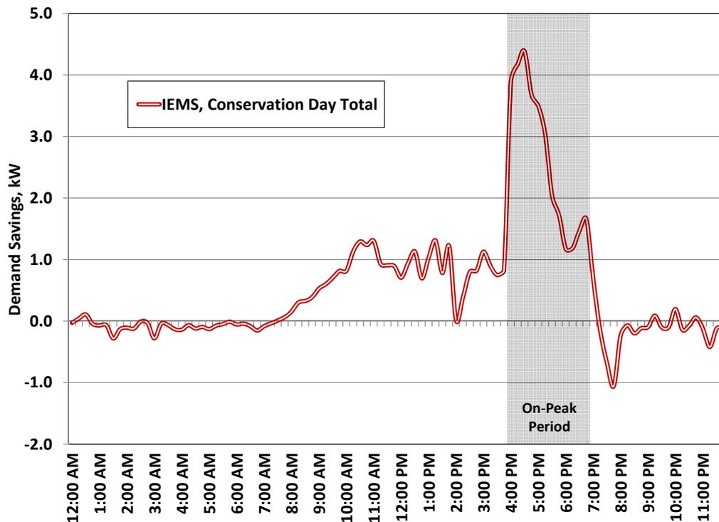
Figure 12 Average House IEMS Total Load Shifting Savings Profile for Conservation Days.
