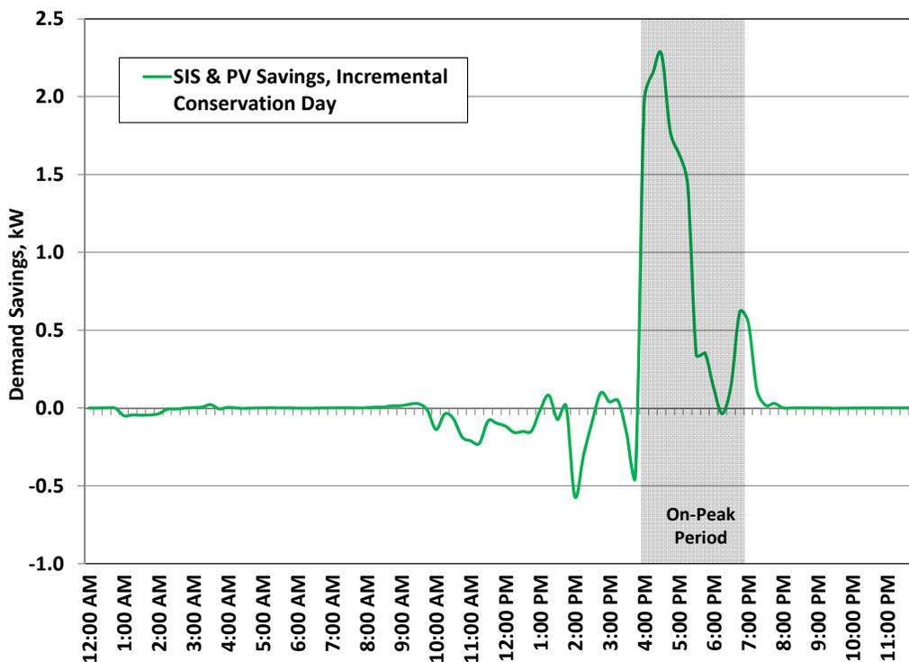
Figure 14 Average House SIS & PV Load Shifting Savings Profile for Incremental Conservation Days.
