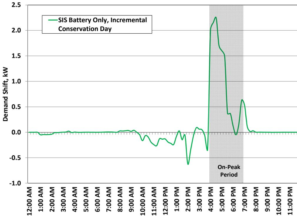
Figure 19 Average House SIS Battery Only Load Shifting Demand Profile for Incremental Conservation Days.
