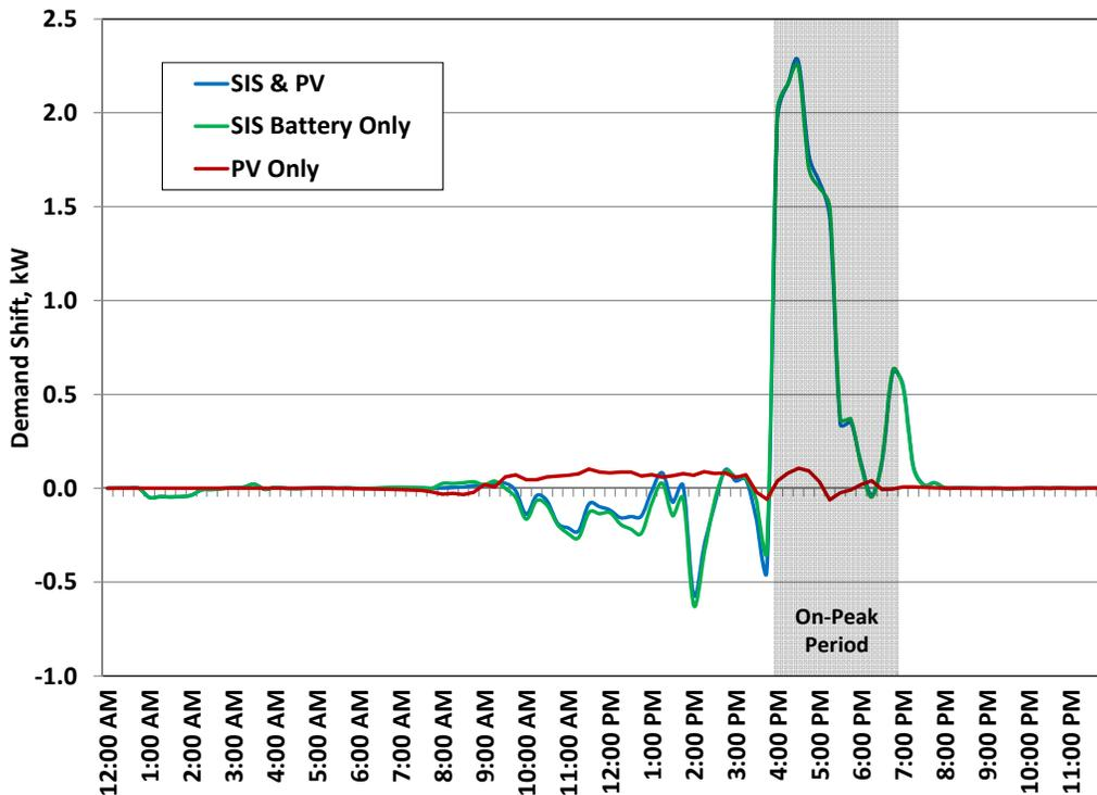
Figure 20 Comparing Incremental Load Shifting Demand Profile for Conservation Days.
