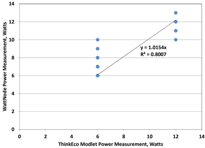
Figure 43 Comparison of WattNode versus Modlet Power Measurements of a Printer.
