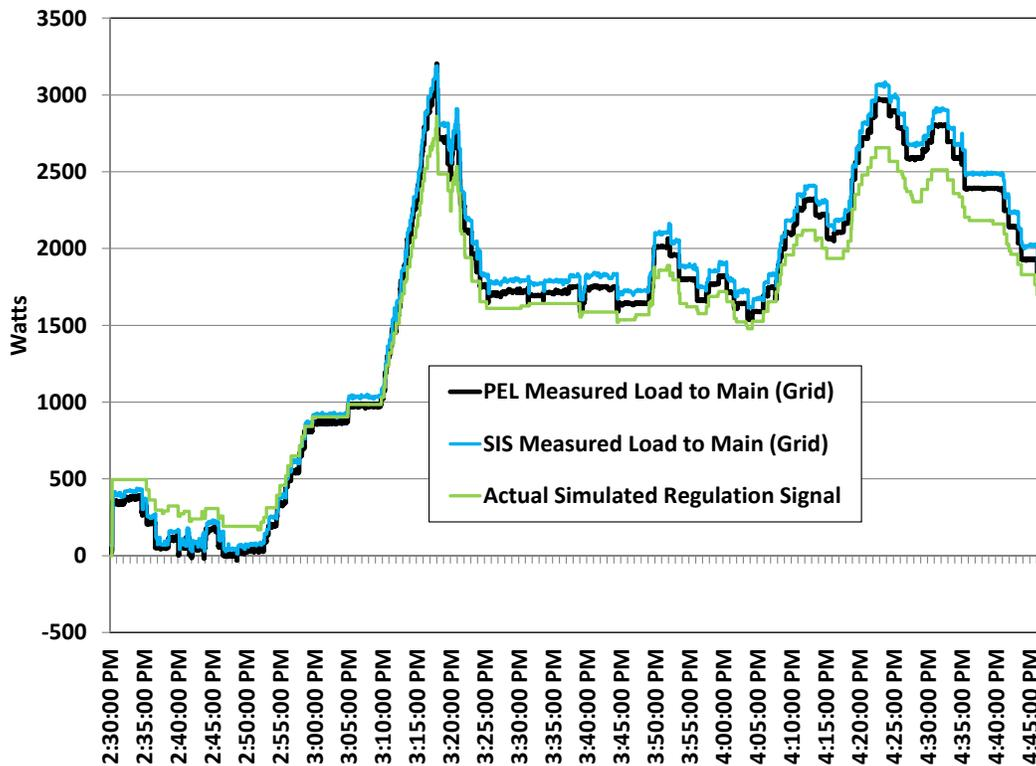
Figure 35 Regulation Test Loads for One SIS Unit.
