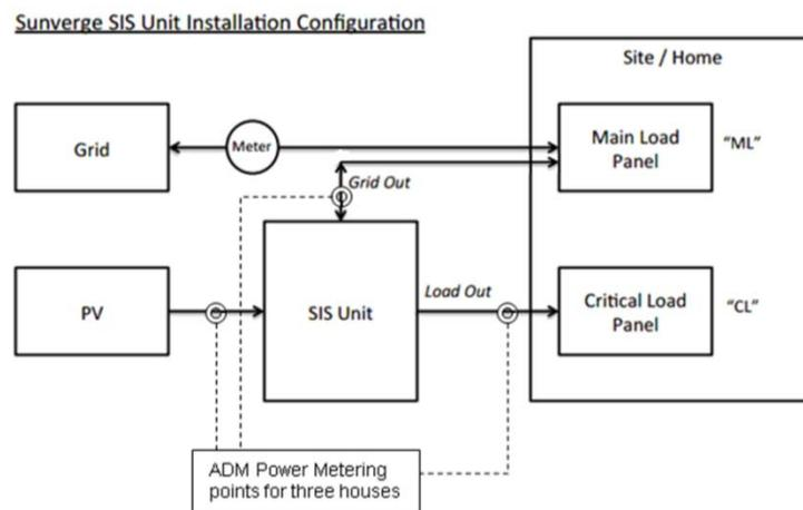
Figure 30 Configuration of Power Meters Installed by ADM at Three Houses.
