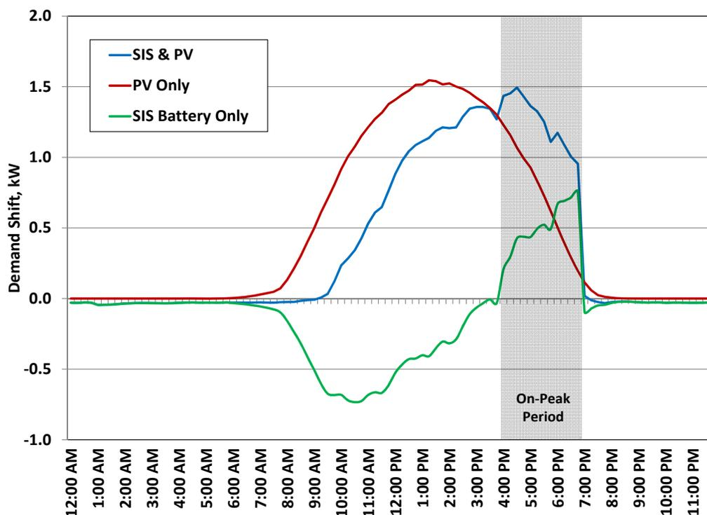
Figure 18 Comparing Load Shifting Profile for Non-Conservation Weekdays.
