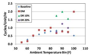
Figure 35. Equipment Cycles per Unit per Hour versus Temperature at JAL Properties
