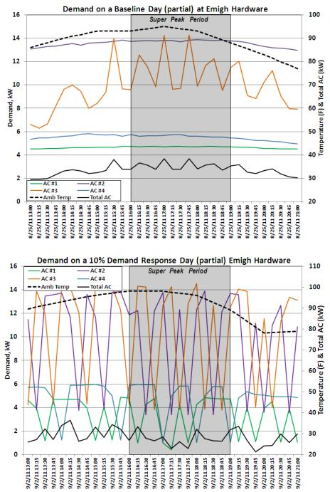
Figure 7. Emigh Hardware – AC Unit Profiles for Baseline and 10% DR Days
