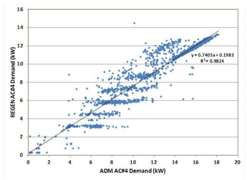
Figure 48. AC#4 at Gold's Gym Natomas Comparison of REGEN to ADM Demand Measurements.
