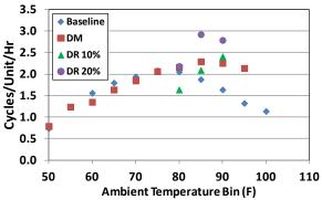
Figure 34. Equipment Cycles per Unit per Hour versus Temperature at Maita Chevrolet
