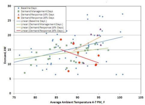
Figure 25. Maximum Peak 15-Minute Demand from 4PM to 7PM at JAL Properties
