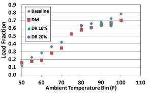
Figure 38. AC Unit Load Fraction versus Temperature at Gold's Gym Elk Grove
