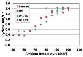
Figure 32. Equipment Cycles per Unit per Hour versus Temperature at Gold's Gym Natomas
