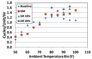
Figure 33. Equipment Cycles per Unit per Hour versus Temperature at Gold's Gym Elk Grove
