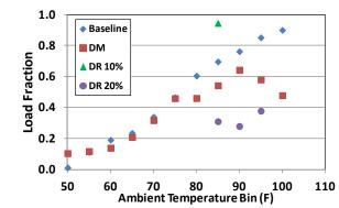
Figure 40. AC Unit Load Fraction versus Temperature at JAL Properties
