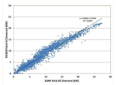
Figure 46. JAL Properties Comparison of REGEN to ADM Demand Measurements.
