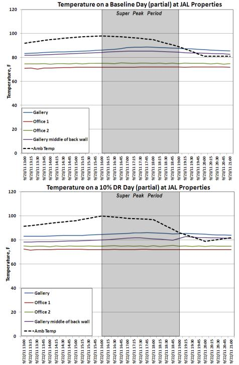
Figure 16. JAL Properties – Temperature Profiles for Baseline and 10% DR days
