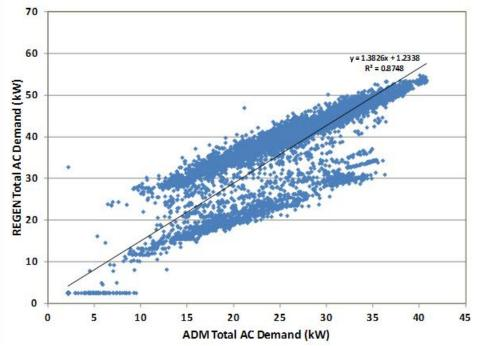
Figure 42. Emigh Hardware Comparison of REGEN to ADM Demand Measurements.
