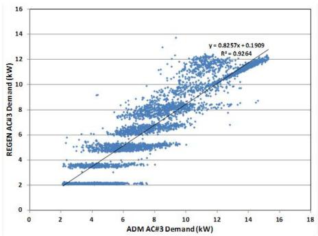
Figure 47. AC#2 at Emigh Hardware Comparison of REGEN to ADM Demand Measurements.
