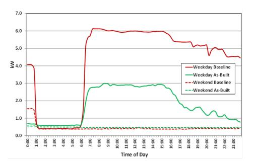
**Figure 12:** Typical weekday and weekend lighting load profiles for the Bimbo Bakery test site. The Evokits and SpaceWise system reduced energy consumption by 49%.
