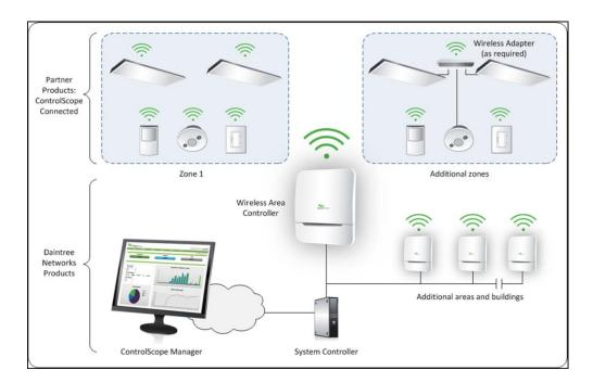
**Figure 6:** The Daintree Networks system uses ZigBee<sup>®</sup>. All of the control devices in the system work to form a wireless mesh network, which helps increase reliability.
