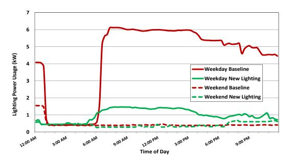
**Figure 7**: The County's project using Philips Evokits and Daintree controls reduced annual lighting energy consumption by 67.9% and peak electrical demand by 71.4% in the tested areas.
