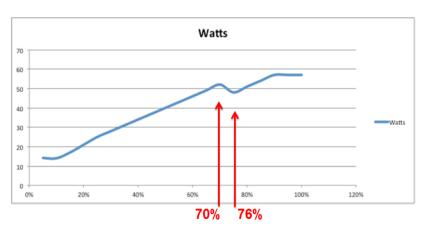
Figure 4: Performance curve for the 0-10V dimming ballast used during the Intel project. Note the power consumption at 76% output is less than at 70%!
