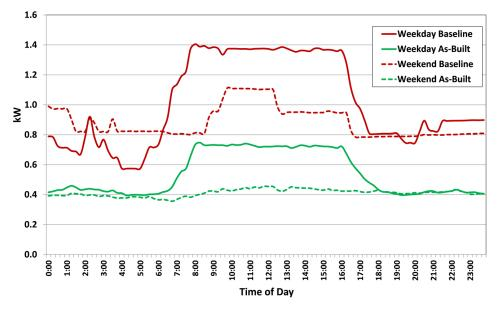
**Figure 13:** Typical weekday and weekend lighting load profiles for the County of Sacramento test site before and after the Evokit/SpaceWise retrofit. The new system reduced energy consumption approximately 49% at this site.
