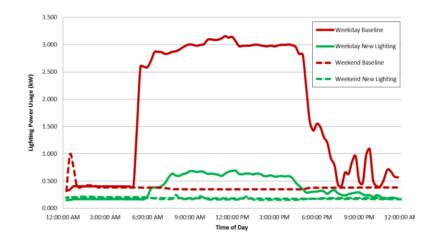
**Figure 20:** County of Sacramento lighting energy profile. The project resulted in energy savings of 76% and a simple payback of 5.7 years (not including labor costs).
