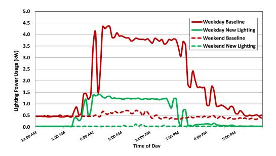
**Figure 9:** Comparison of the typical weekday and weekend lighting load profiles before and after the LG LED Lighting and Daintree controls retrofit. The new system reduced energy consumption by an estimated 75%.
