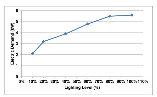
Figure 5-4: Electrical Demand at Various Dimming Levels
