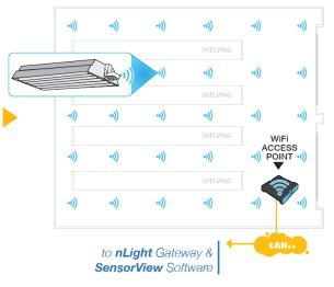
Figure 2-1: nLIGHT Wireless Lighting Controls Source: http://nlightcontrols.com/wpontent/uploads/nwifi\_brochure.pdf
