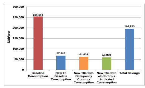
Figure 3-9: Monitored Energy Consumption and Total Savings for the new lighting system and controls
