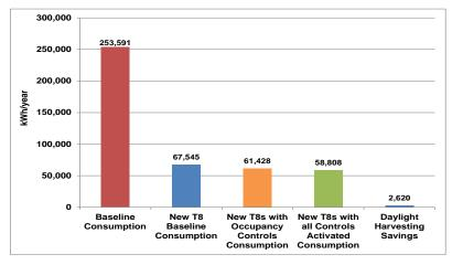
Figure 3-7: Monitored Energy Consumption and Savings with Daylight Harvesting Activated
