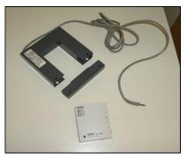
Figure 5-1: Hobo Logger and Current Transducer (CT)
