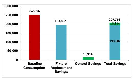
Figure 3-12: Disaggregated Energy Savings from nLIGHT's GreenScreen Software
