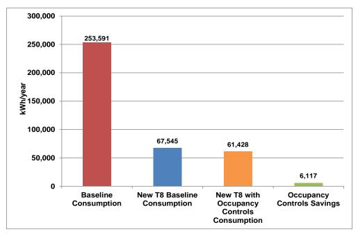
Figure 3-5: Monitored Energy Consumption and Savings with Activated Occupancy Controls
