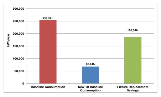
Figure 3-3: Monitored Energy Consumption and Savings with New T8 Fixtures
