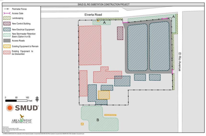
Figure 2-1. Conceptual Substation Plan
