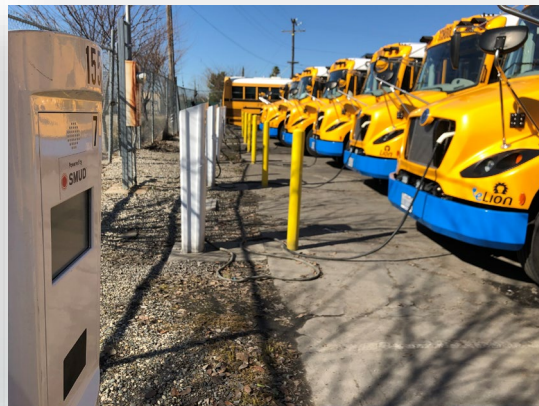
Electric school bus pilot testing vehicle to grid
