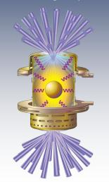
The x-rays blow off the fuel capsule wall, accelerating the fuel inward to 1 million MPH
