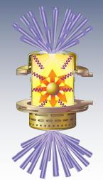
The fuel core reaches 100 times the density of lead and ignites at 100,000,000°C
