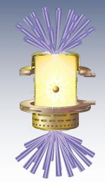
Fusion burn spreads rapidly through the compressed fuel, yielding many times the input energy
