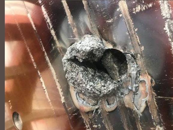
Through bolt through lamination
