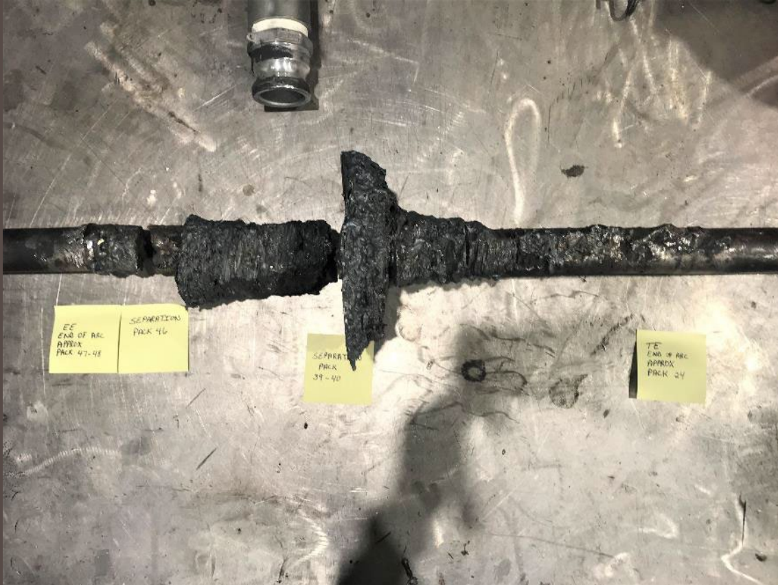
Through Bolt following removal
