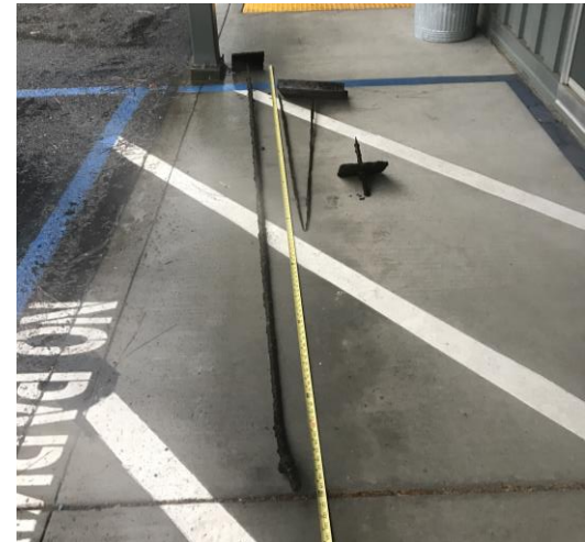
Bottom: Recovered rock bolts
