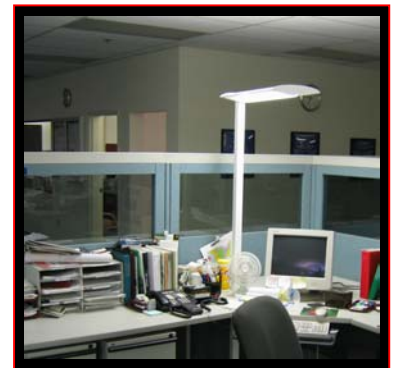
Using only task lights can create a cave effect. Note the dark walls when only the task light is on.
