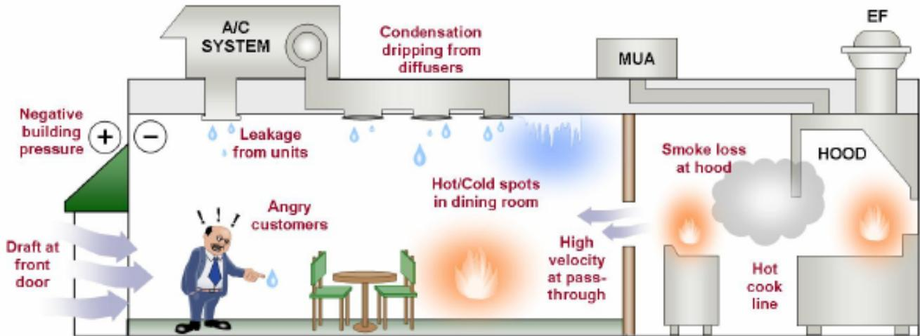
**Figure 1:** Unbalanced ventilation systems waste energy and may cause a variety of comfort and air quality problems that affect both customers and staff. Drawing provided courtesy of Melink Corporation.
