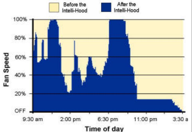
**Figure 2:** This graph shows the fan speeds for a ventilation system equipped with Melink's Intelli-Hood controls. Note that the fans run at part speed the majority of the time. Source: Melink Corporation.
