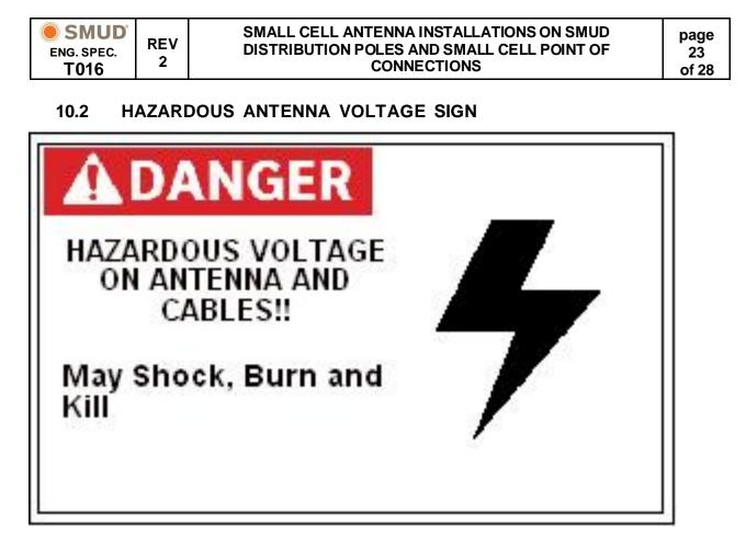
Make sign from 18-gauge steel with Porcelain Enamel finish, Red "Danger" header with all other copy and symbols black on white background, size 8.5" x 14", 4 holes with 1/2" i. d. brass grommets, located 1/2" in from each corner, (Standard Sign Blank).
