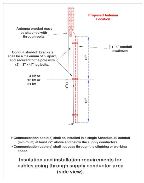
This drawing is to show the clearance requirements of the conduit openings with respect to the primary conductors. Actual construction and conduit attachments in the field may vary depending upon the location and the equipment being installed.
