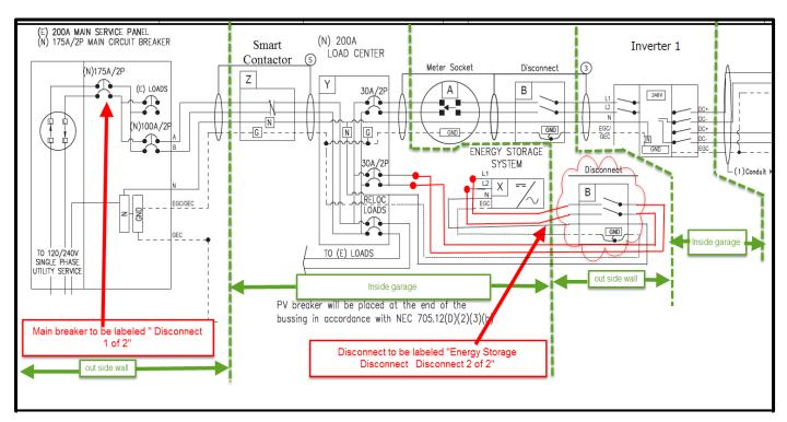
Figure 4 – The drawing above (from Tesla) shows an example of an additional disconnect, its location, and labeling, which would be required if the ESS is located in a garage.
