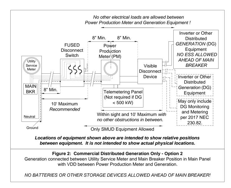
7.2. Commercial – DG only, No ESS – Option 2: Generation connected between Utility Service Meter and Main Breaker position as per applicable NEC code. A FUSED Disconnect Switch needs to be installed between the Main Panel and the Power Production Meter (2017 NEC 230). All other items from 7.1.2 through 7.1.8 (except 7.1.5) apply.
