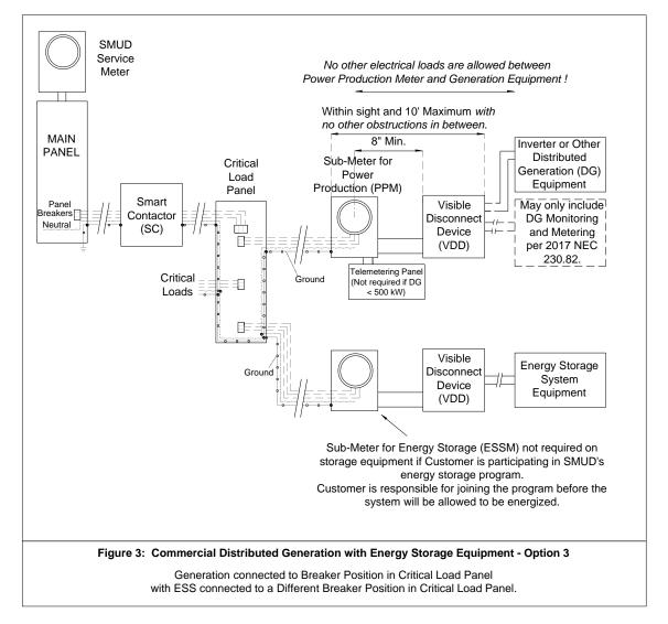
7.3.1. As with previous options, there can be no other load between the Power Production Meter and the DG equipment, other than loads necessary for the monitoring and metering of the DG equipment.
