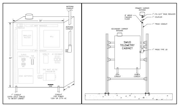
Figure 7 - Equipment Layout Figure 7a- Physical Cabinet Elevation (SMUD will install the equipment)
