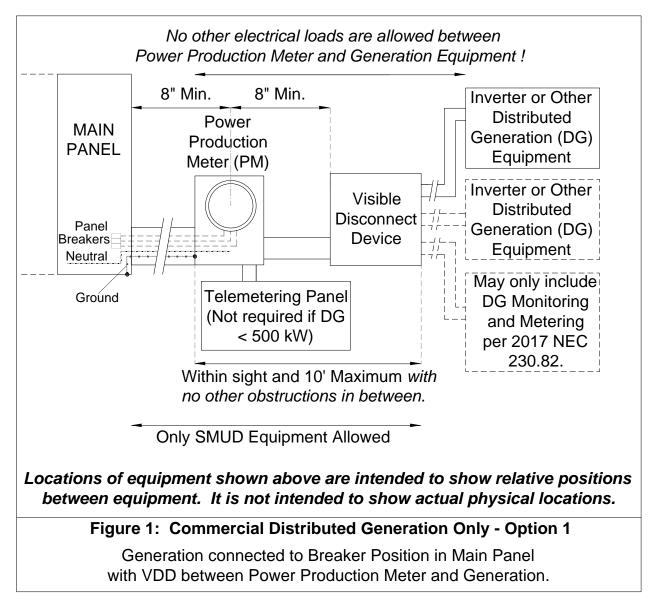
7.1. **Commercial – DG only, No ESS – Option 1:** Generation connected to a breaker position in Main panel located at the opposite end of the bus from the Main breaker or otherwise located per applicable NEC code.
