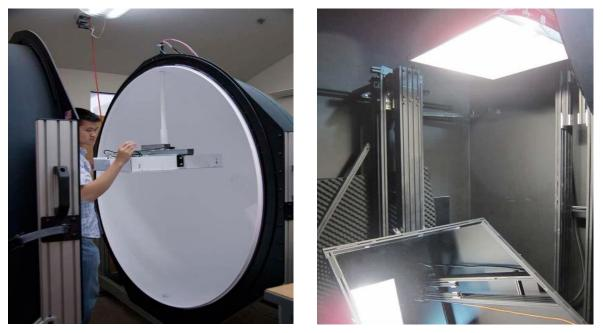
Figure 7: Integrating Sphere (left) and Goniophotometer (right)
