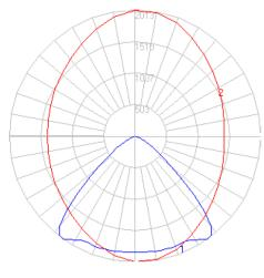
Vertical Plane Through Horizontal Angles: Blue: 90° - 270° (Through Max Candela)
