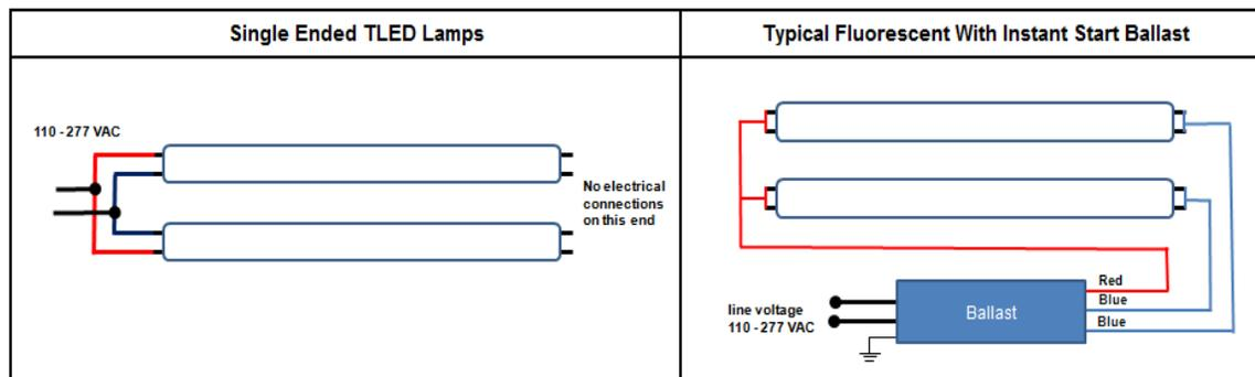
Figure 2: Fixture Wiring
