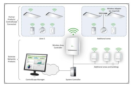
Figure 5: Daintree's wireless mesh network
