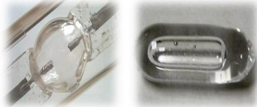
**Figure 3:** Conventional metal halide lamps require electrodes within the arc tube—a potential failure point. LEP does not require the use of electrodes.
