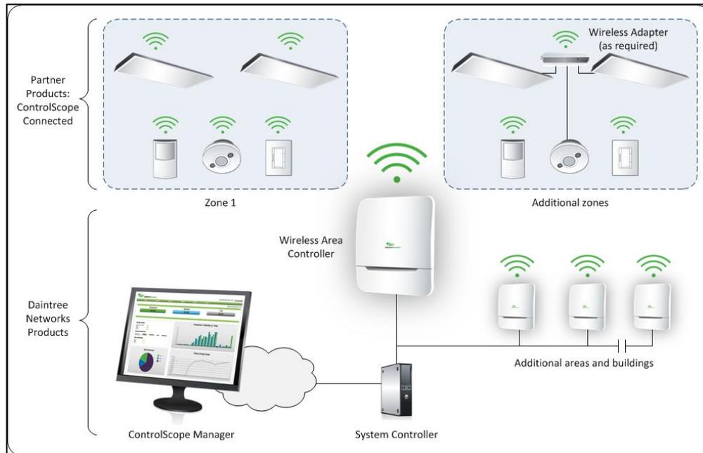
**Figure 5:** Daintree's wireless mesh network
