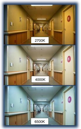
**Figure 7:** The new hallway fixtures were controlled via automatic controls for both dimming and Kelvin-changing.
