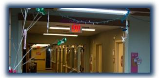
**Figure 16:** The new LED hallway lights significantly reduced the amount of glare and use 70% less energy than the fluorescent fixtures they replaced.
