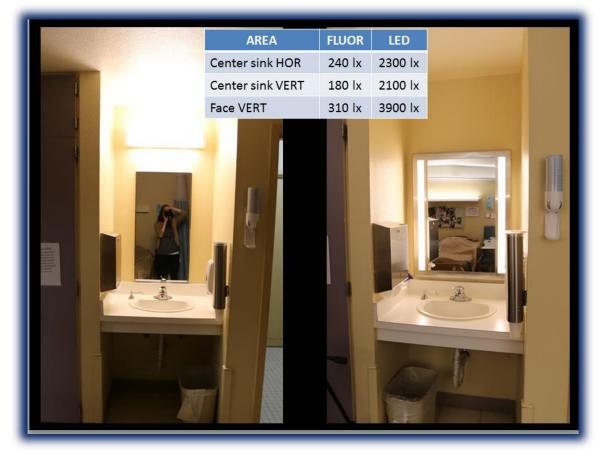
The LED light levels here were measured with the fixture at its maximum output. The levels shown far exceed what is needed, but the fixture would usually be used at a dimmed setting.
