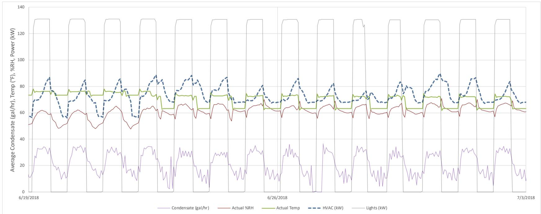
Figure 15. Additional Trend Data for Room B – increasing relative humidity possibly due to increasing plant transpiration
