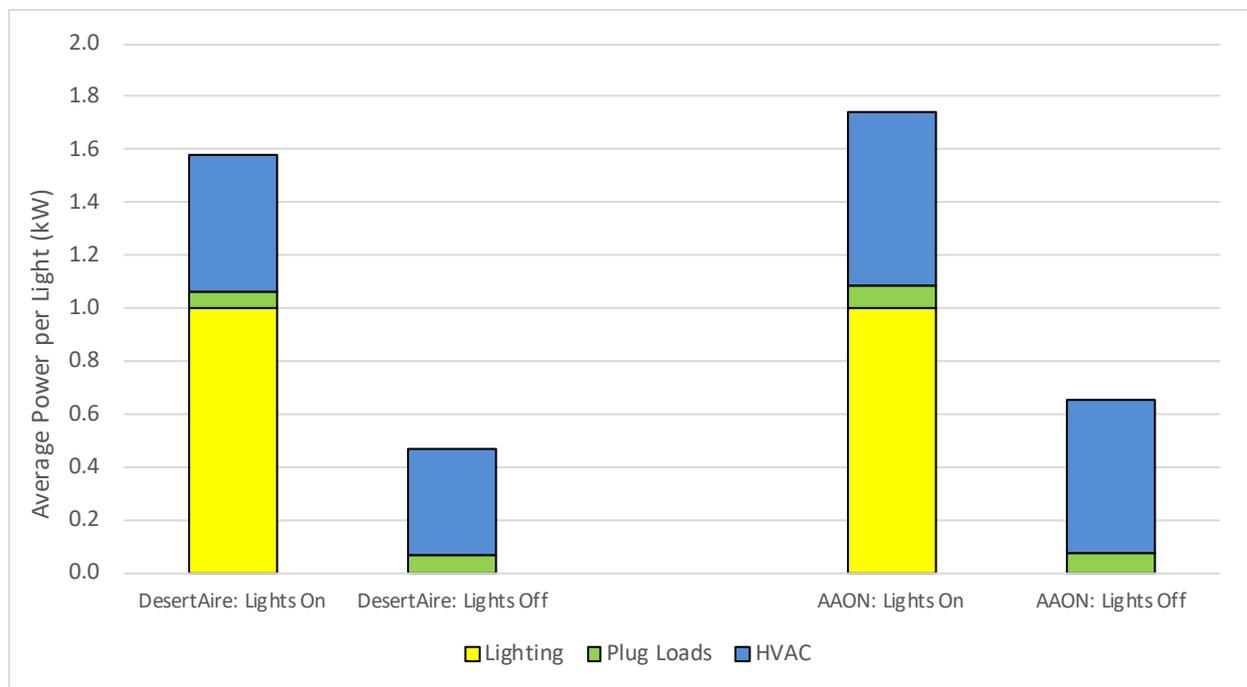
**Figure 3.** Comparison of Rooms in On/Off Mode: Average HVAC and Plug Power per 1,000-Watt HPS Light During Flowering Stage
