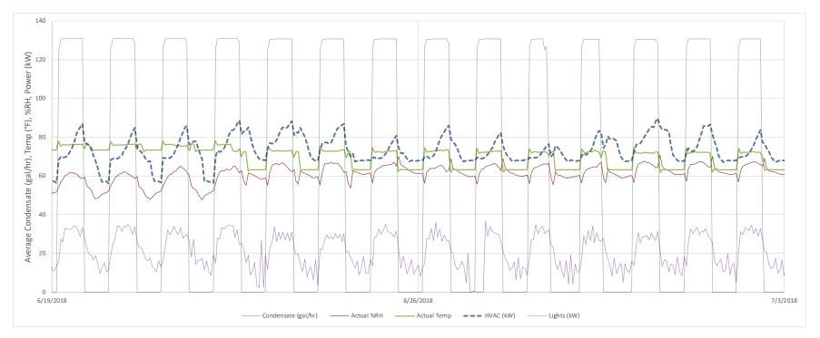
Figure 15. Additional Trend Data for Room B – increasing relative humidity possibly due to increasing plant transpiration
