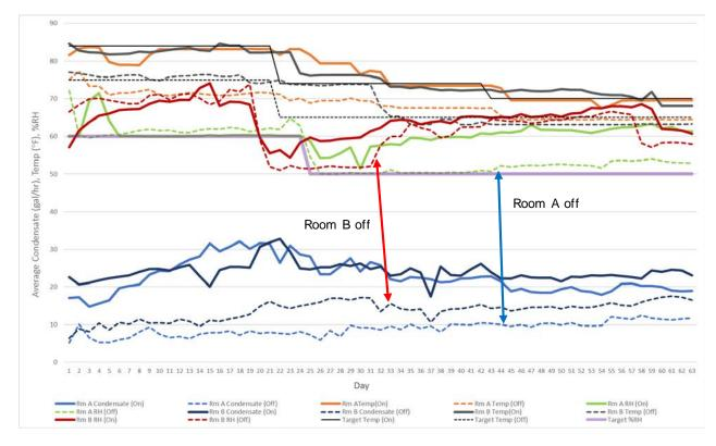
**Figure 6.** Trending Daily Average Setpoints and Actual Conditions for Both Grow Rooms \*Note\* Condensate rate in Room B was reduced by the ratio of plants in Room A to Room B to make a more direct comparison
