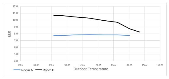
Figure 9. EER versus Outdoor Temperature for Room A and Room B Systems
