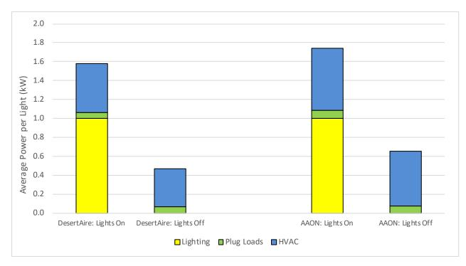
Figure 3. Comparison of Rooms in On/Off Mode: Average HVAC and Plug Power per 1,000-Watt HPS Light During Flow ering Stage
