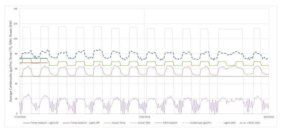
Figure 12. Room A grow cycle – Showing relative humidity % is no longer maintained when lights are off
