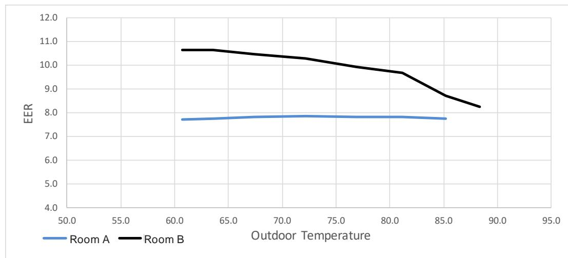
**Figure 9.** EER versus Outdoor Temperature for Room A and Room B Systems
