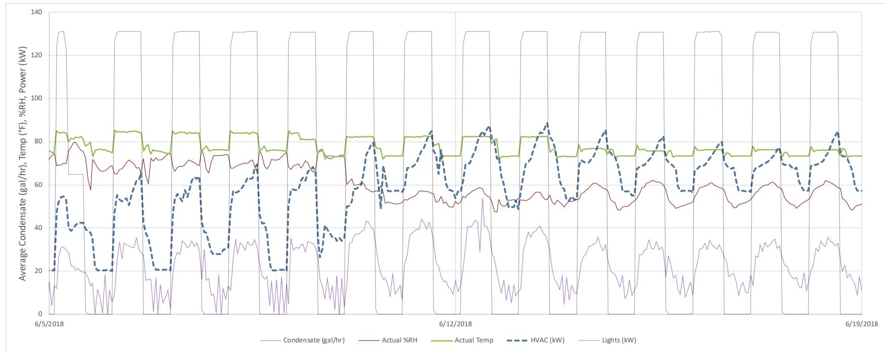
**Figure 14. Additional Trend Data for Room B – Weeks 3 and 4 (temperature setpoint change from 84 to 74 when lights are on and 75 to 65 when lights are off)**
