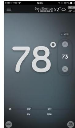
During testing there were connectivity problems with the thermostat about every hour – an issue that was not apparent for other thermostats. The only way to reset the Wi-Fi connection is to power the unit off.
