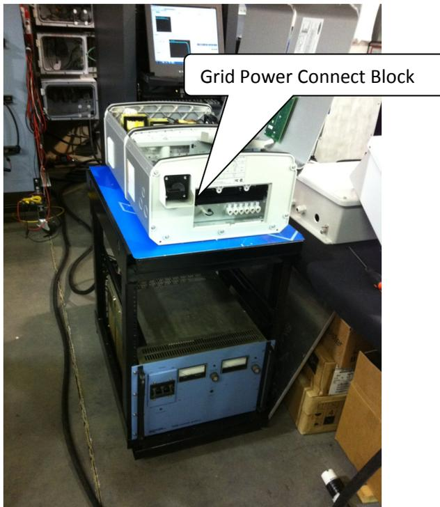
**Figure 4-4. Inverter and DC power supply**
