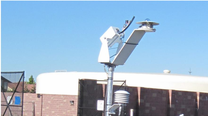
**Figure 6-8. One of the four RSRs with a PSP installed**
