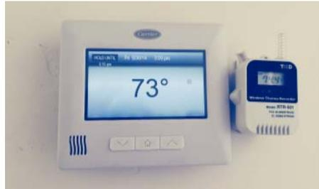
*Figure 8 Wireless Temperature Logger Mounted Next to Carrier Thermostat (PCT).*
